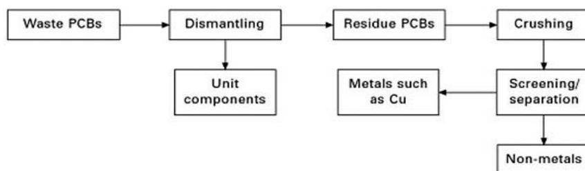
Fig. 1. Scheme of mechanical processing of waste printed circuit boards; scheme developed based on [58].
