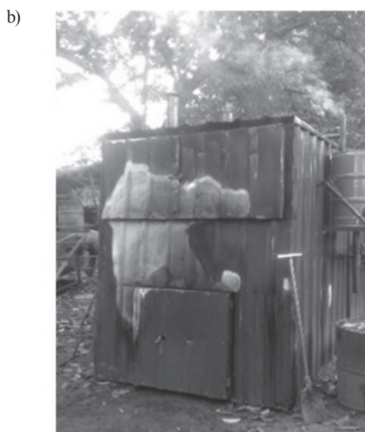
Fig. 2. Smoke produced by: a) conventional method, b) tar scrubber pyrolysis reactor.
