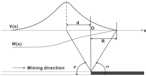
Fig. 2. Calculation coordinate system of surface dynamic subsidence.
