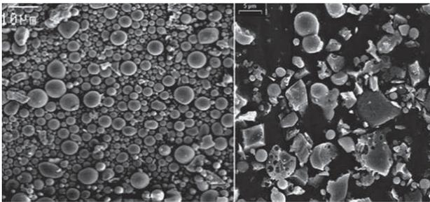
Fig. 4. Fly ash microstructure with 10 μm and 5 μm particle.
