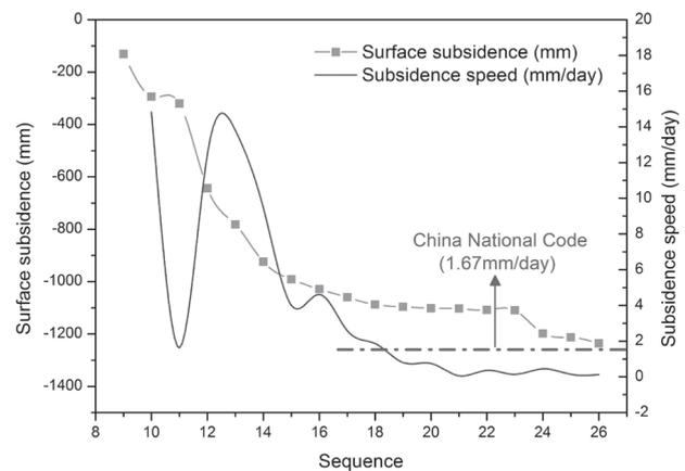
Fig. 5. Surface subsidence and subsidence speed curves of no. 17 point.
