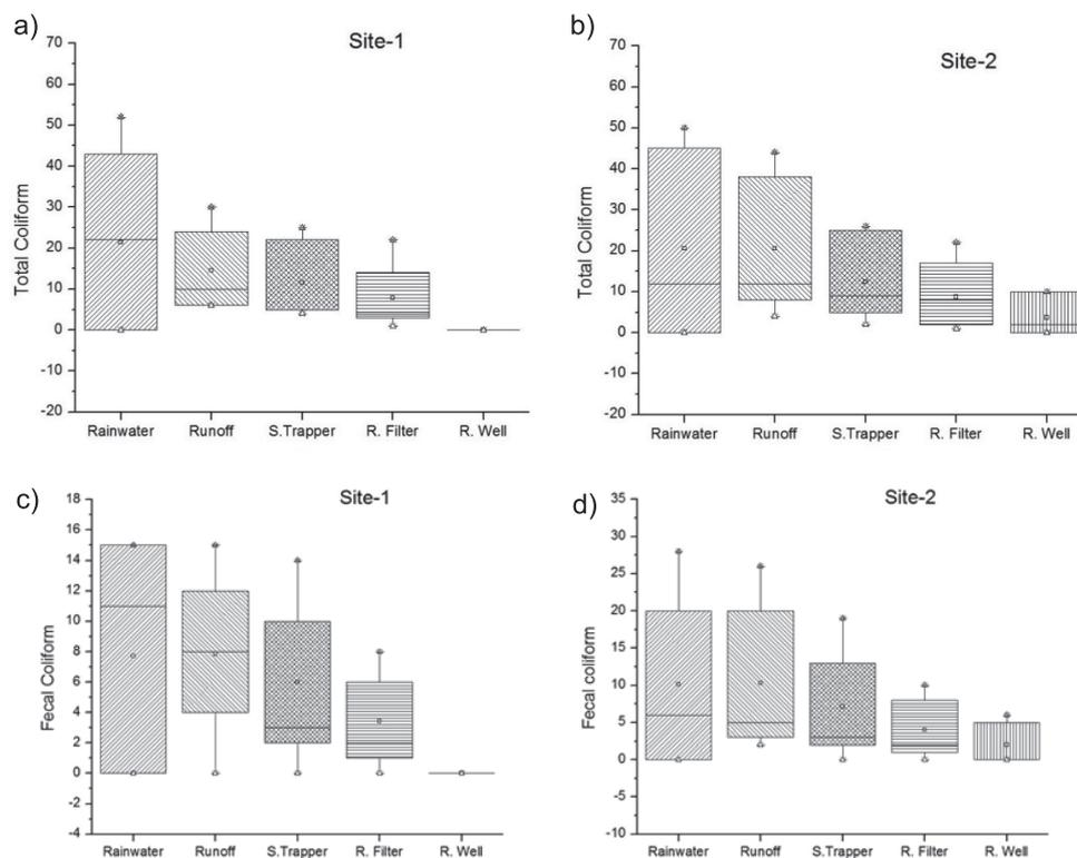
Fig. 10. Monthly average values of total coliform and fecal coliform of rain water at various filtration blocks of artificial recharge wells at PCRWR and STEDEC.
