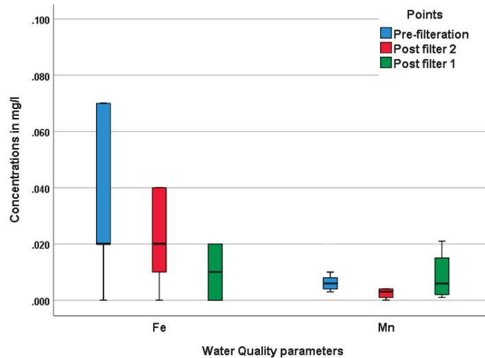
Fig. 5. Comparing Fe and Mn pre-and post-filtration.
