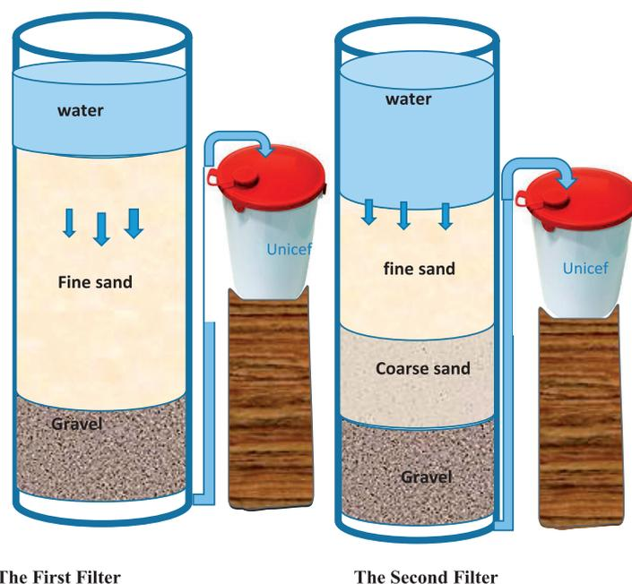
Fig. 1. An illustration of the two designed filters.
