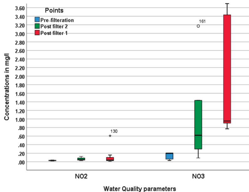
Fig. 6. Comparing NO<sub>2</sub> and NO<sub>2</sub> pre-and post-filtration.
