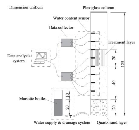
Fig. 2. Schematic diagram of test device.
