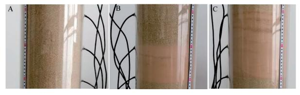
Fig. 3. Test treatment design of soil columns. A: CK, no loess layer; B: LS, containing loess at 40-50 cm and sand at 50-60 cm; C: LL, containing loess at 40-60 cm.
