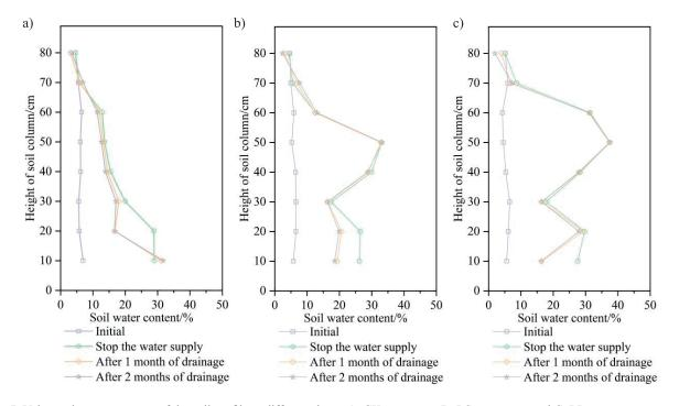
Fig. 7. Volumetric water content of the soil profile at different times. A, CK treatment; B, LS treatment; and C, LL treatment.
