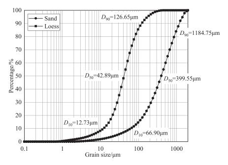
Fig. 1. Grain size distribution curves of sand and loess.
