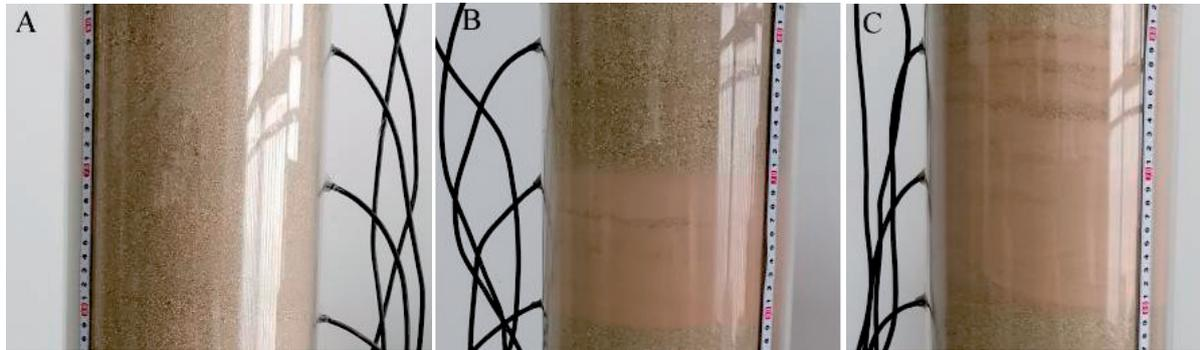
Fig. 3. Test treatment design of soil columns. A: CK, no loess layer; B: LS, containing loess at 40-50 cm and sand at 50-60 cm; C: LL, containing loess at 40-60 cm.
