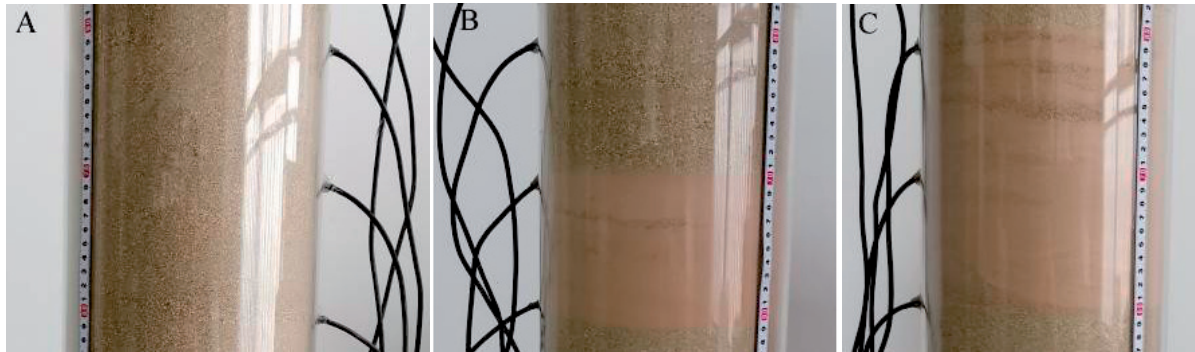
Fig. 3. Test treatment design of soil columns. A: CK, no loess layer; B: LS, containing loess at 40-50 cm and sand at 50-60 cm; C: LL, containing loess at 40-60 cm.
