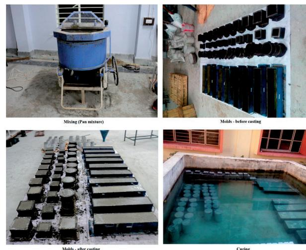
Fig. 2. Mixing, casting and curing of HPC.
