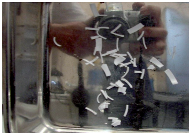
Fig. 2. Polystyrene adhering to the metal surface of the cuvette.
