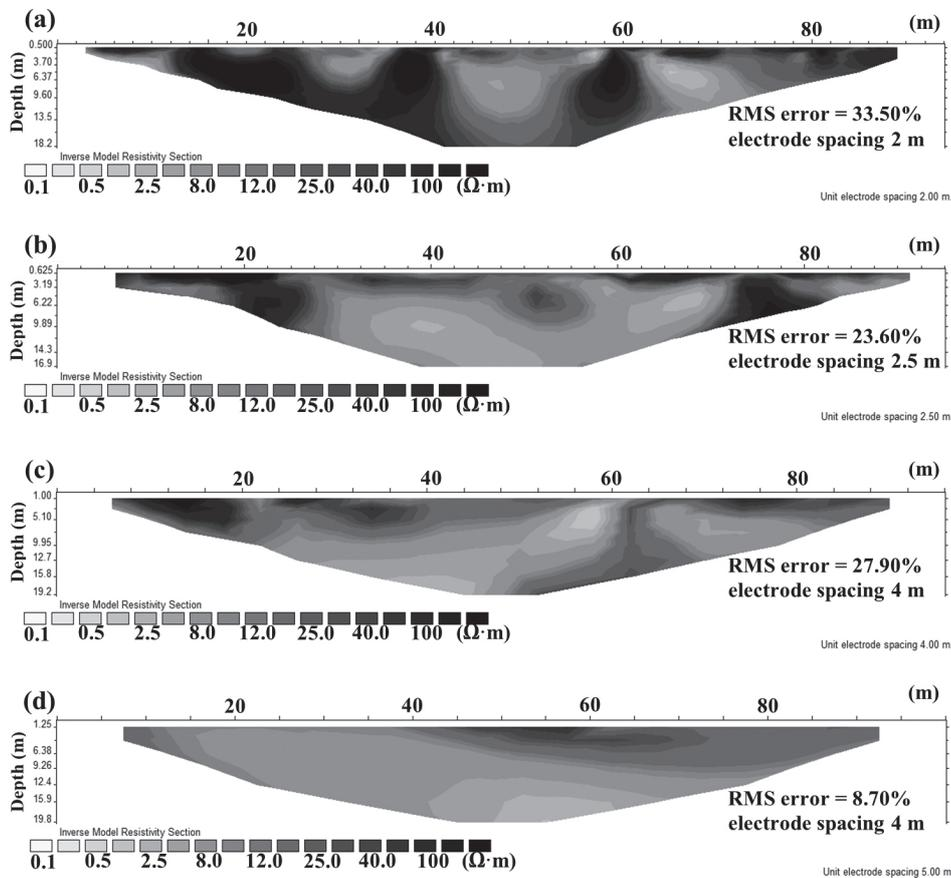
Fig. 8. True resistivity inversion models of the apparent resistivity data from surveying with spacing values of a) 2 m, b) 2.5 m, c) 4 m, and d) 5 m.
