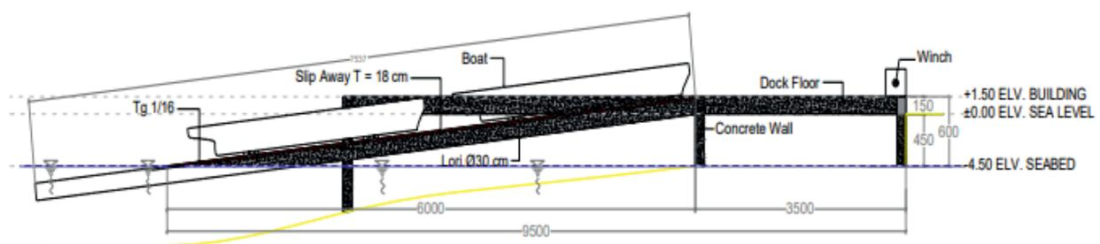
Fig. 3. Slipways (in mm).
