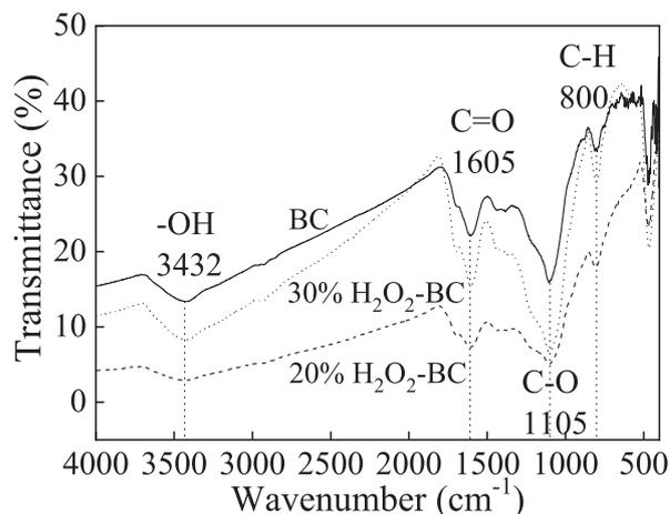
Fig. 1. Fourier transform infrared spectrum of rice husk-derived biochar before and after H<sub>2</sub>O<sub>2</sub>-modification.
