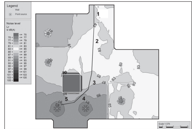
Fig. 2. The distribution of the acoustic field – variant 1. Using this solution one can obtain complete information about the area in which the employee is located and his or her logistics over the course of a normal working day. Markings 1-5 are indexes of sections of sample trajectory.
