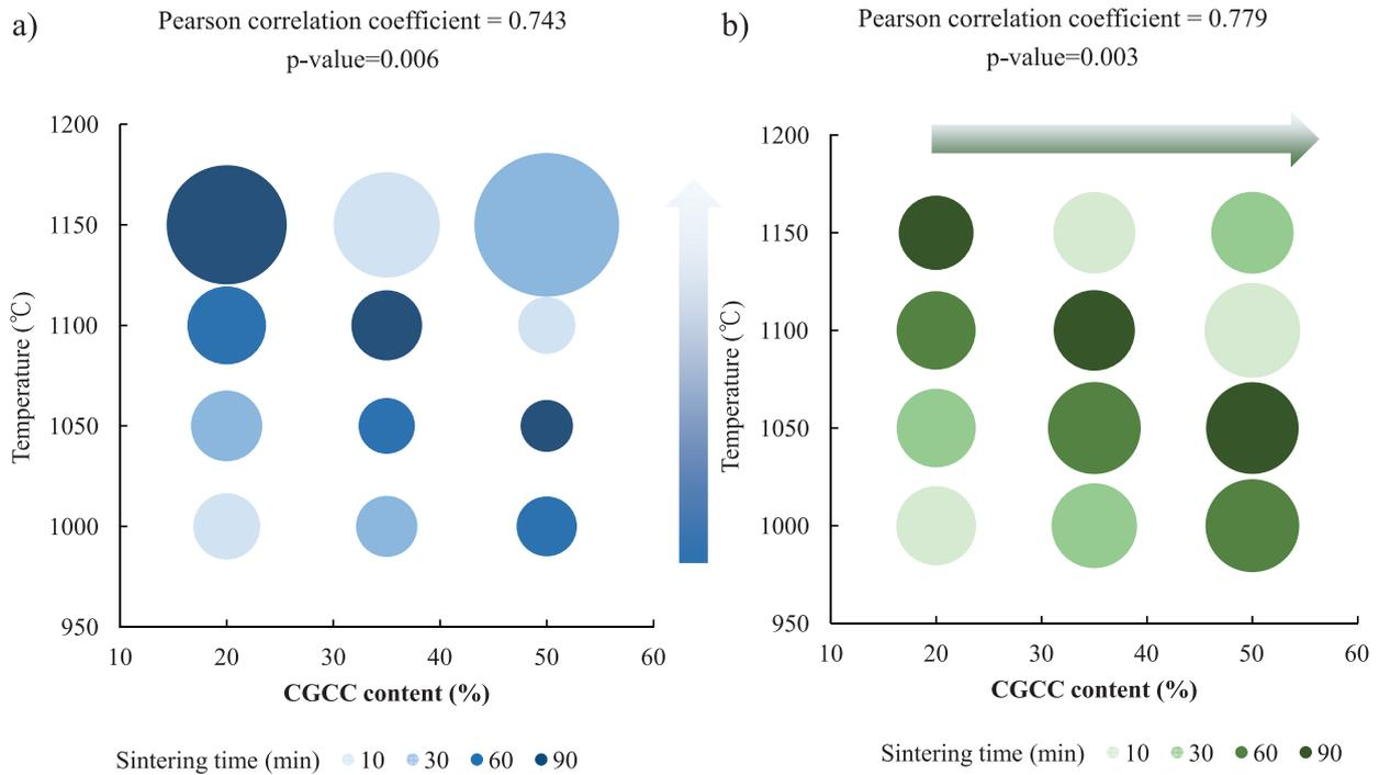
Fig. 2. Ceramsite compressive strength a) and water absorption b). The diameter of the air bubble is positively correlated with compressive strength or water absorption, and the various shades represent different sintering times.
