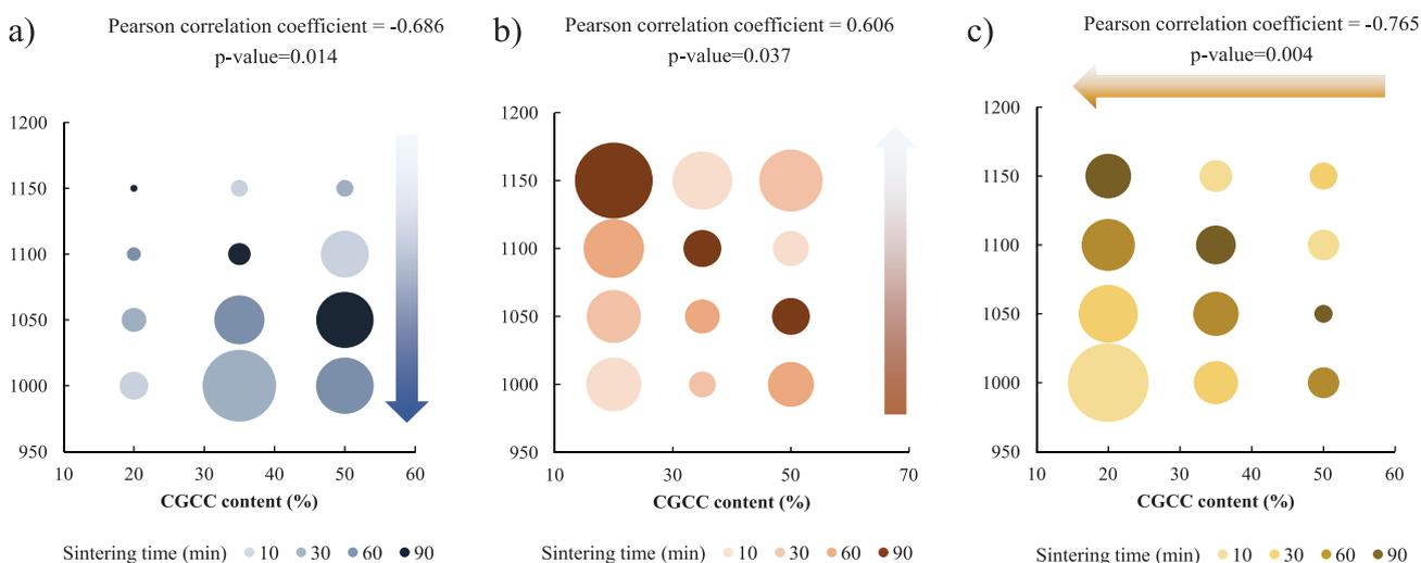
Fig. 3. The leaching toxicity of ceramsite as Cr a), As b), and Hg c). The diameter of the air bubble is positively correlated with the concentrations of trace elements (Cr, As, and Hg), and the various shades represent different sintering times.
