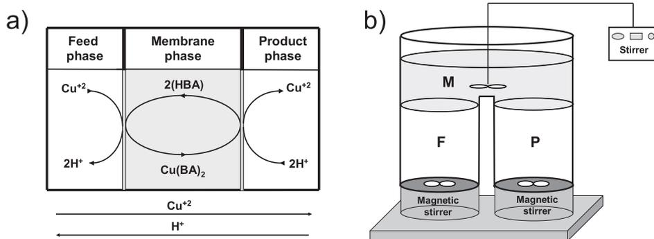
Fig. 1. a) Diagram of the facilitated countertransport of Cu(II) ions using HBA as carrier and  $\text{H}^+$  as counter ions, b) Schematic representation of the experimental cell (F, feed phase; M, membrane phase; P, product phase).
