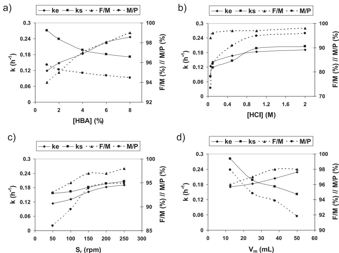
Fig. 2. Influence of different parameters on the removal/recovery kinetic constants ( $k_e$ ,  $k_s$ ) and on the transport efficiencies through feed/membrane (F/M) and membrane/product (M/P) interfaces: a) benzoylacetone concentration in membrane phase, b) hydrochloric acid concentration in product phase, c) stirring rate, d) membrane phase volume.
