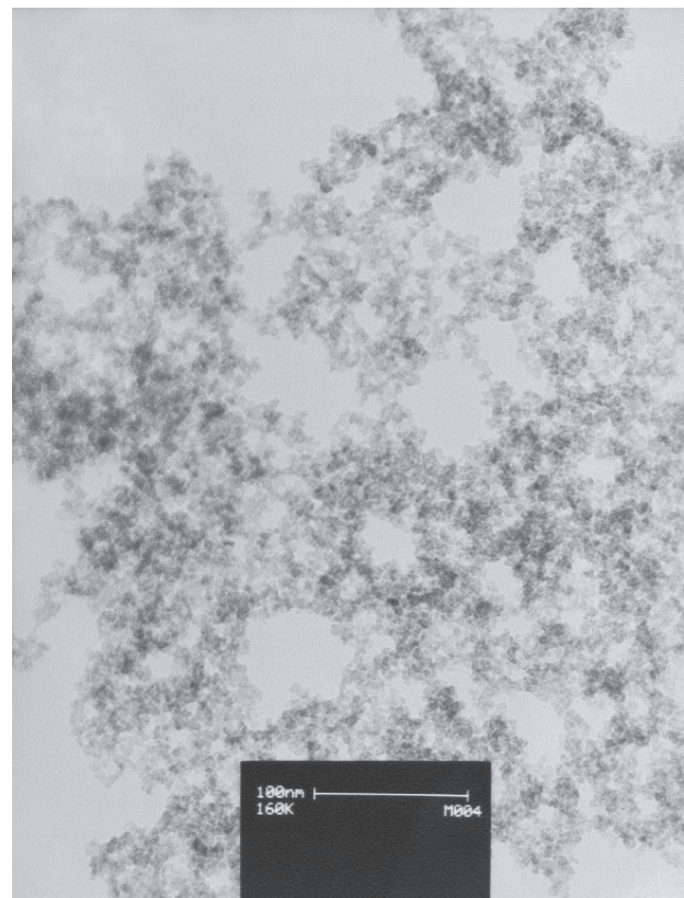
Fig. 3. TEM images of ZnO NPs 160 K magnification at a scale of 100 nm
