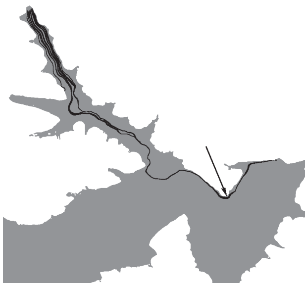
Fig. 8. Particle tracking for Dobczyce Reservoir from Wolnica Creek inlet to the dam outlet (average annual discharge, no wind); arrow denotes the position of the water supply inlet.
