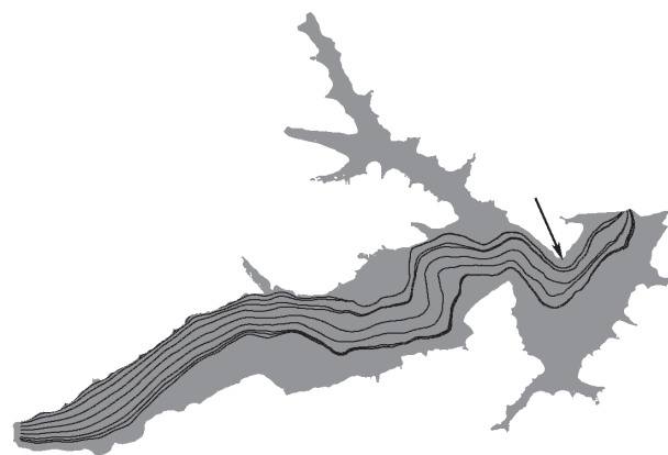
Fig. 6. Particle tracking for Dobczyce Reservoir from the Raba River inlet to the dam outlet (average annual discharge, no wind); the arrow denotes the position of the water supply inlet; the current-driven particles reach the inlet about 3 days after entering the reservoir.
