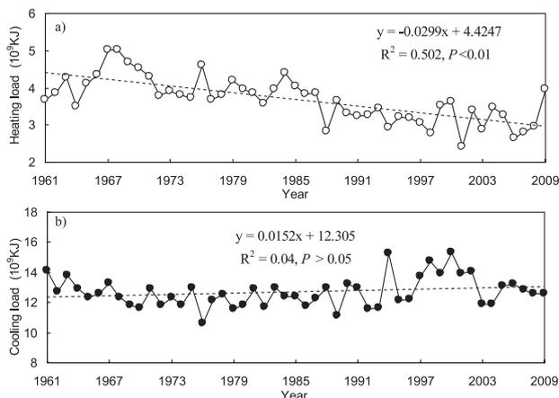
Fig. 2. Interannual variations in energy load for heating a) and cooling b) in commercial buildings, 1961-2009.
