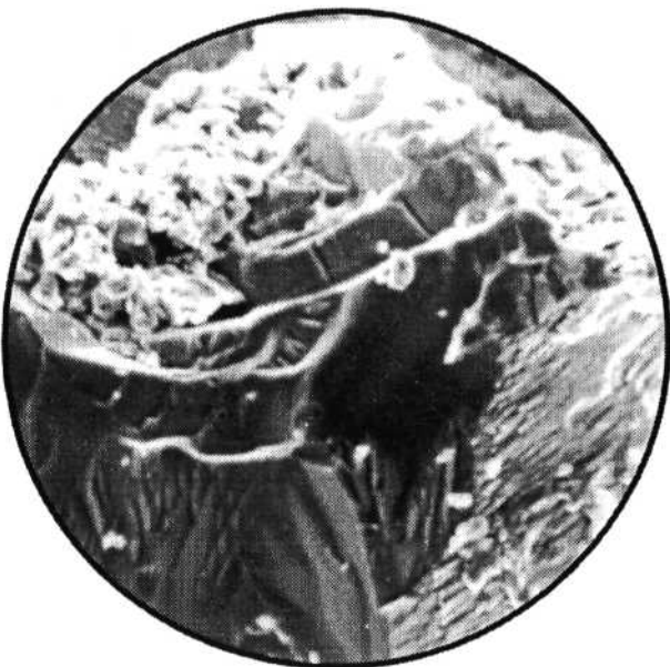
Photo 2. Chalcopyrite (0.16-0.12 mm grain size) after leaching
