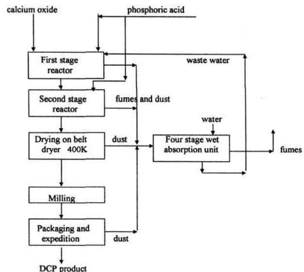
Fig. 3. Low-temperature exothermic DCP production process realized on new unit.
