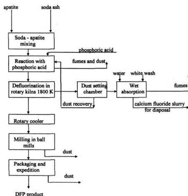
Fig. 1. Conventional thermal method of the DFP production process.
