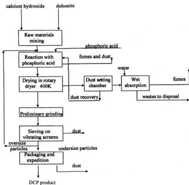
Fig. 2. Low-temperature endothermic DCP production process realized on DFP unit.
