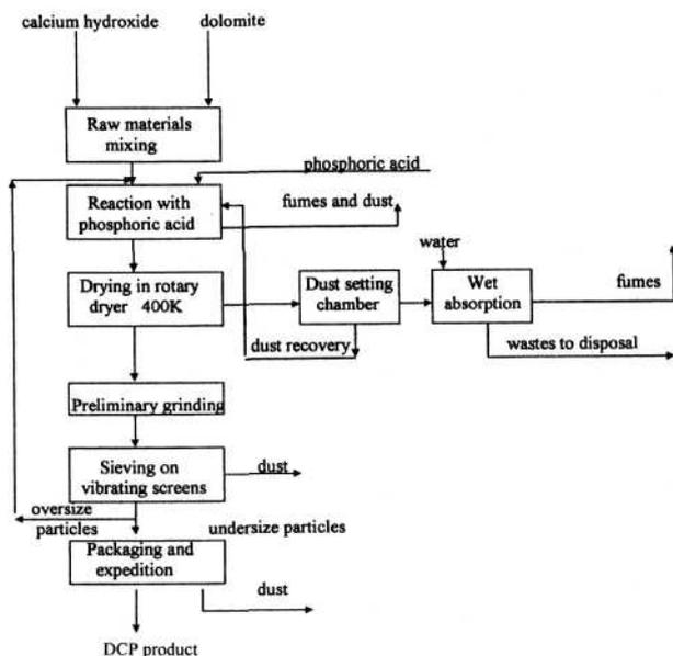
Fig. 2. Low-temperature endothermic DCP production process realized on DFP unit.
