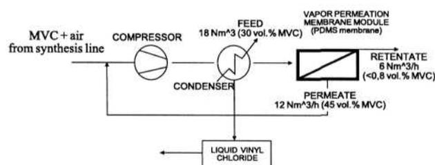
Fig. 20. Flow diagram of compression/condensation and membrane separation for MVC recovery [39].
