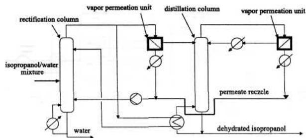
Fig. 11. Isopropanol dehydration by combined vapor permeation and above-azeotropic distillation [51].
