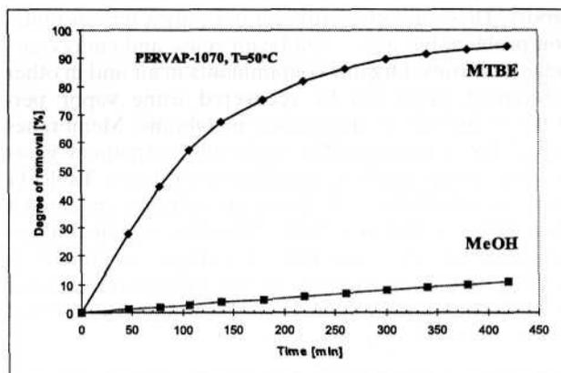
Fig. 16. Batch mode pervaporation. Removal of MTBE and MeOH from water using PERVAP-1070 membrane. Feed volume to membrane area ratio  $120 \text{ dm}^3/\text{m}^2$ . Initial organics concentration: MeOH: 2%, MTBE:1%.
