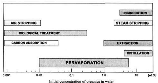
Fig. 15. Comparison of the separation methods for VOCs removal from water [39].
