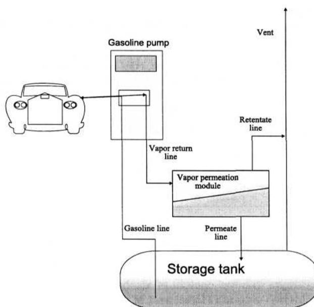
Fig. 19. Flow scheme of GKSS vapor return system [46].
