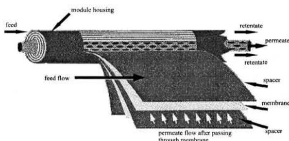
Fig. 5. Schema of a spiral-wound module.
