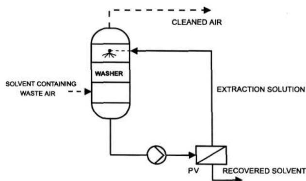
Fig. 18. Removal of solvents from waste air [37, 39].
