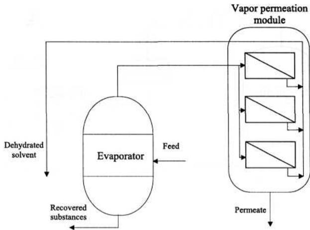
Fig. 13. Flow diagram of a hybrid process consisting of an evaporator followed by vapor permeation module for solids recovering and liquids recycling [45].
