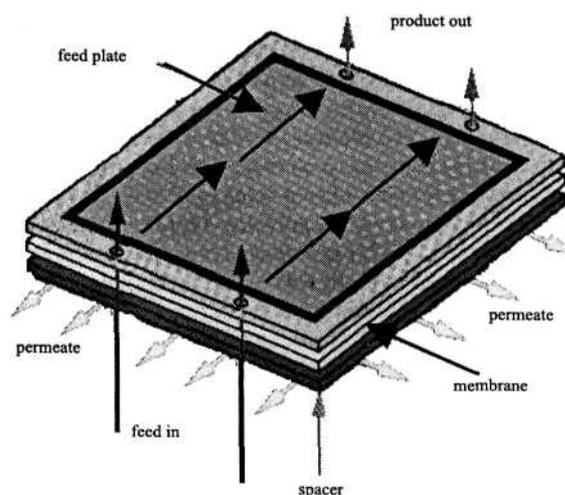
Fig. 4. Schema of a plate-and-frame module.
