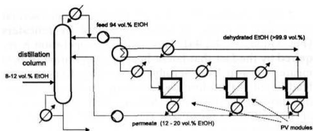
Fig. 10. Schema of the dehydration of ethanol by distillation-pervaporation hybrid process.
