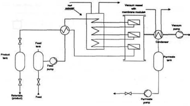
Fig. 7. Schema of a pervaporation plant.
