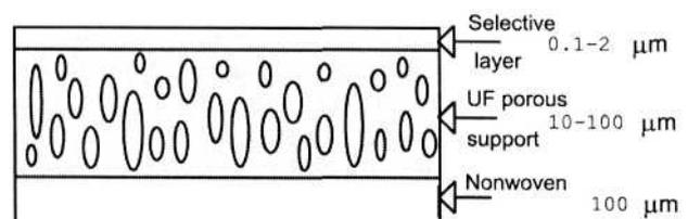
Fig. 3. Morphology of the pervaporation composite membrane.
