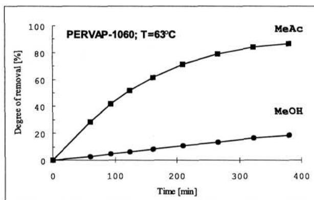
Fig. 17. Batch mode pervaporation. Removal of MeAc and MeOH from water using PERVAP-1060 membrane. Feed volume to membrane area ratio  $120 \text{ dm}^3/\text{m}^2$ . Initial organics concentration: MeOH: 6.4%, MeAc: 1.6%.
