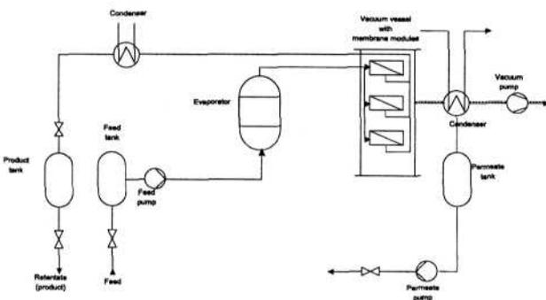
Fig. 8. Flow chart of the vapor permeation unit.
