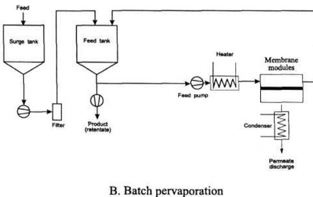
Fig. 9. Possible operation modes of pervaporation.
