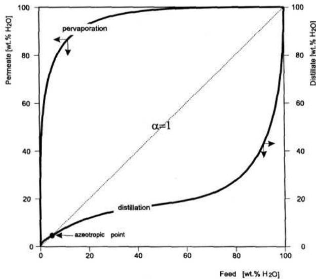
Fig. 2. McCabe-Thiele separation diagram. Comparison of pervaporation selectivity with distillation selectivity. System: water-ethanol. Membrane: PVA composite hydrophilic membrane.
