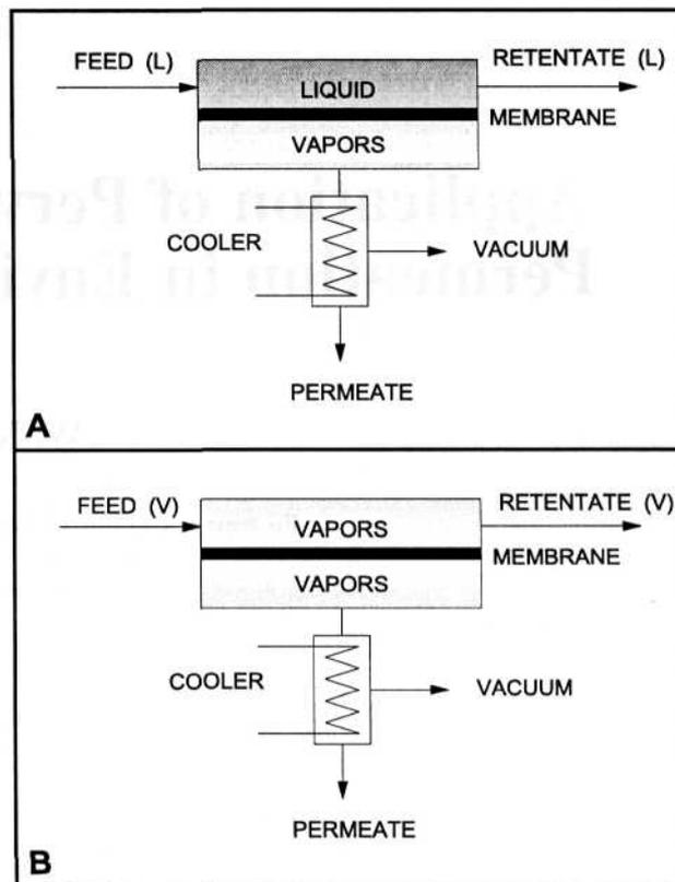
Fig. 1. Schema of pervaporation (A) and vapor permeation (B) processes.
