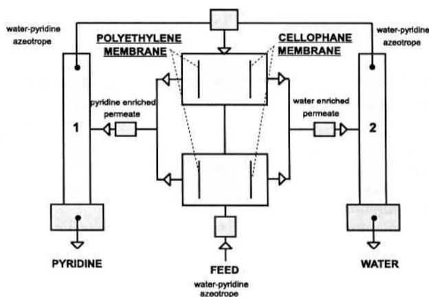
Fig. 6. Schema of the distillation-pervaporation process for the dehydration of water-pyridine azeotrope (according to Binning) [40].
