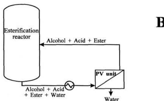
Fig. 12. Pervaporation enhanced synthesis of esters.
