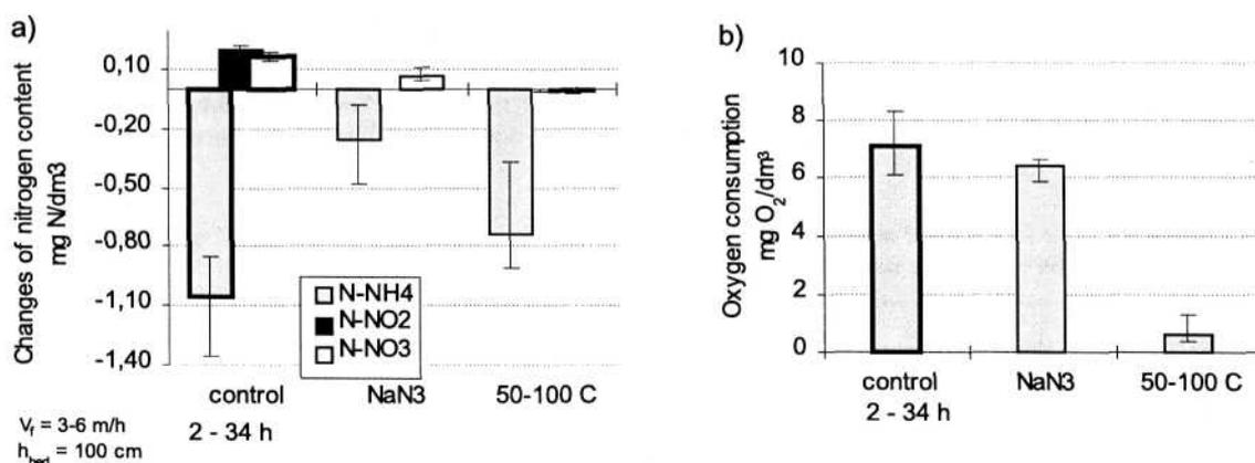
Fig. 3. Changes of contents of various forms of mineral nitrogen (a) and oxygen consumption (b) during the I-st stage filtration on the mature sand filter before and after inhibiting microbial activity.
