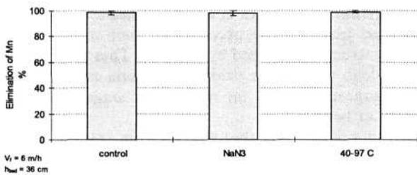
Fig. 4. Efficiency of manganese elimination during the II-nd stage filtration on mature sand filter before and after inhibiting microbial activity by intoxicating the bed with  $\text{NaN}_3$  and by treating the bed with high temperature.
