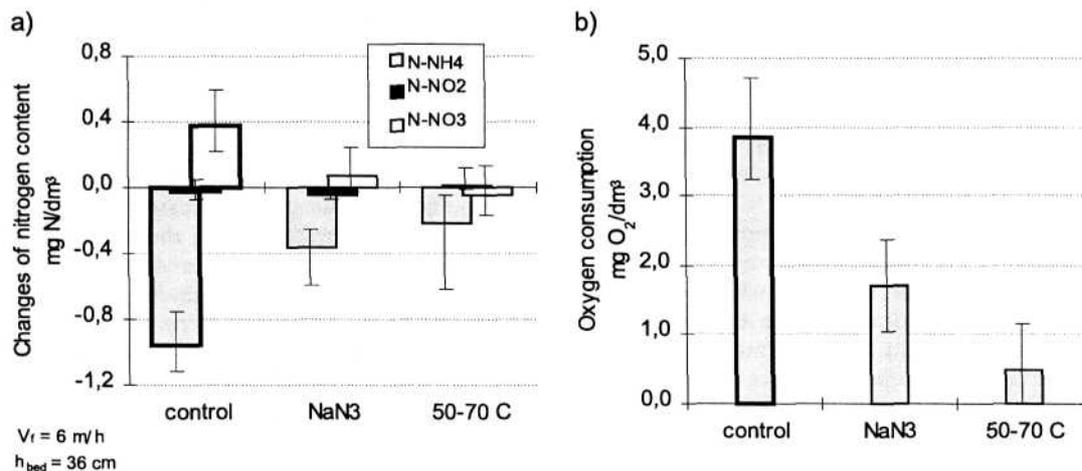
Fig. 5 Changes of contents of various forms of mineral nitrogen (a) and oxygen consumption (b) during the II-nd stage filtration on the mature sand filter before and after inhibiting microbial activity.
