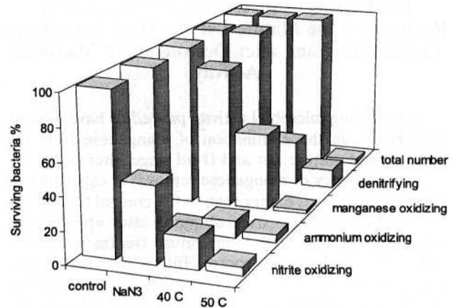
Fig. 1. The percentage share of bacteria surviving on the sand bed after intoxication with 15 mM  $NaN_3$  and after treatment at 40°C and 50°C.
