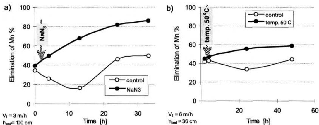
Fig. 2. Efficiency of manganese elimination during the I-st stage filtration on mature sand filter before and after inhibiting microbial activity by intoxicating the bed with  $\text{NaN}_3$  (a) and by treating the bed with high temperature (b).
