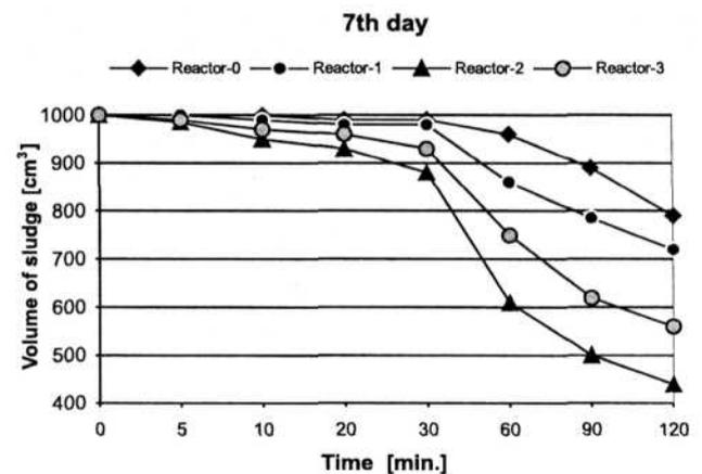
Fig. 6. Variation of settling characteristics during aerobic digestion - 7<sup>th</sup> day.
