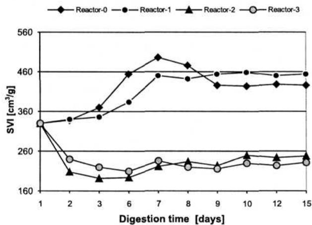
Fig. 4. SVI changes during aerobic digestion in the presence of H<sub>2</sub>O<sub>2</sub> and Fenton's reagent.
