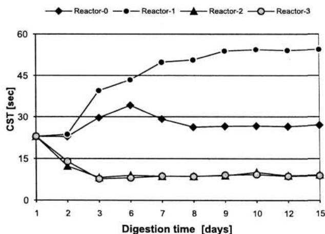
Fig. 3. CST changes of sludge during aerobic digestion in the presence of  $H_2O_2$  and Fenton's reagent.
