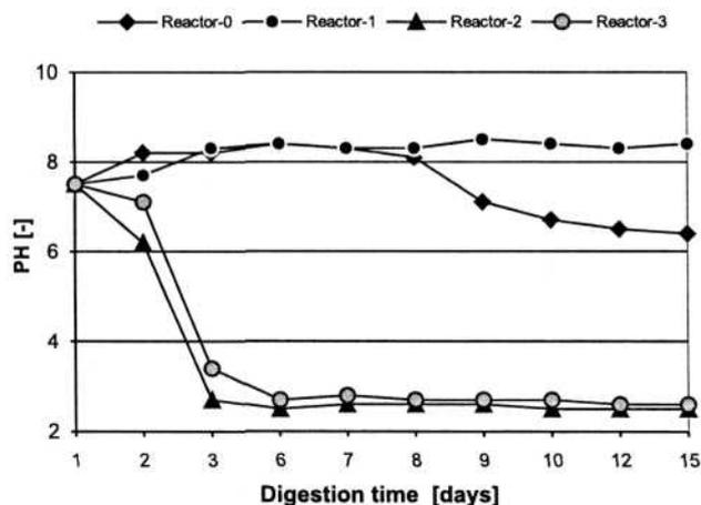
Fig. 2. pH changes in the R-0 + R-3 reactors during aerobic digestion in the presence of  $H_2O_2$  and Fenton's reagent.
