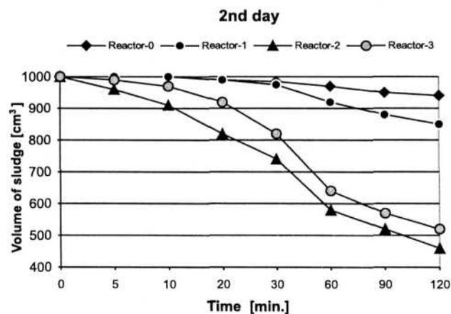
Fig. 5. Variation of settling characteristics during aerobic digestion - 2<sup>nd</sup> day.
