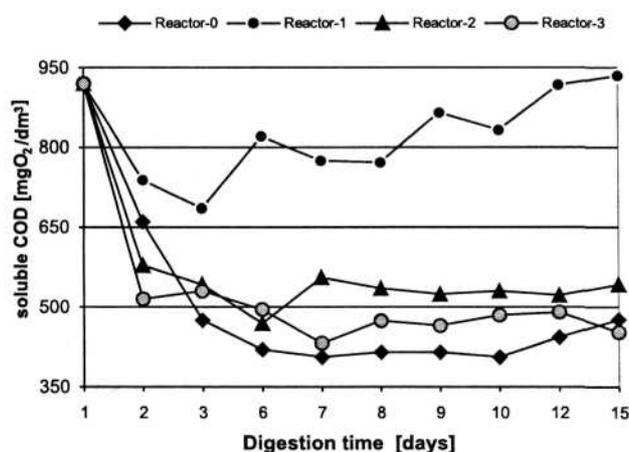
Fig. 1. COD changes for supernatants during aerobic digestion in the presence of H<sub>2</sub>O<sub>2</sub> and Fenton's reagent.
