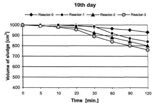
Fig. 7. Variation of settling characteristics during aerobic digestion - 10<sup>th</sup> day.
