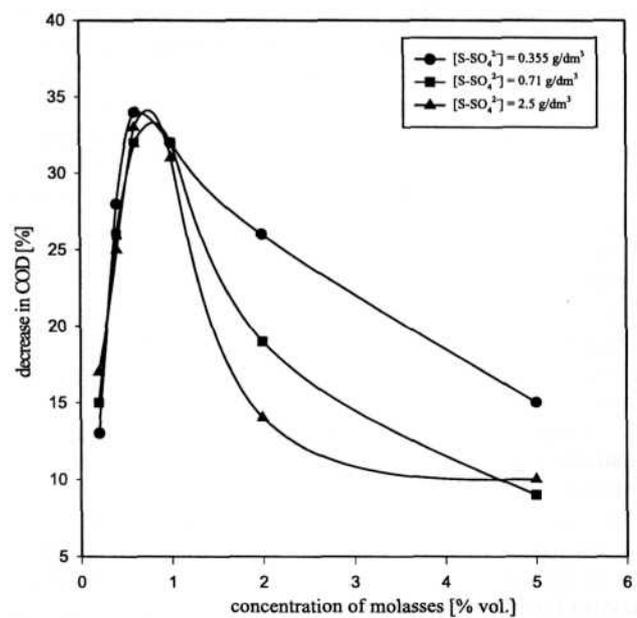
Fig. 2. A decrease in COD in percent, in the media with different concentrations of SO<sub>4</sub><sup>2-</sup> and molasses (temp. 37°C, pH = 7, *Desulfotomaculum ruminis* bacteria)
