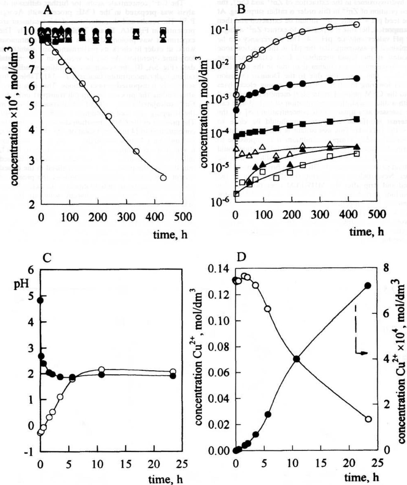
Fig. 5. Continuous membrane extraction (CME) (A, B) and diffusion dialysis (C, D) process for the recovery and concentration of Cu(II). Concentration vs. time dependence for metal extraction (A) from the feed and re-extraction (B) into the stripping solution: (•) Zn, (o) Cu, (■) Ca, (□) Mg, (▲) Na, (△) K. Diffusion dialysis of the Cu concentrate: changes in pH (C) and Cu concentration (D) in the concentrate (o) and acid stripping solution (•).
