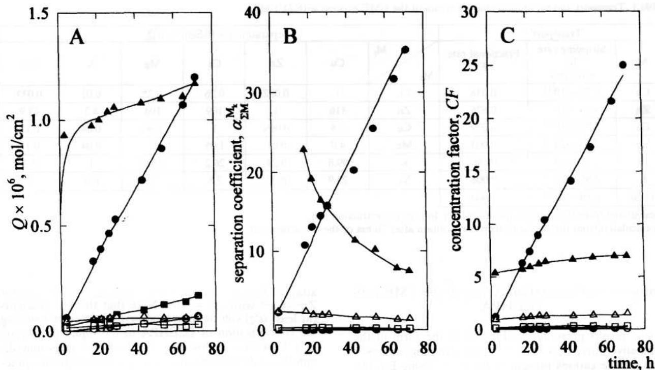
Fig. 3. Transport properties of the CME system with D2EHPA: (A) cumulative stripping curves, (B) overall separation coefficients, (C) concentration factors;
