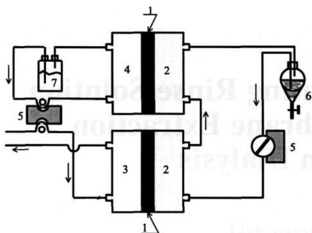
Fig. 1. Scheme of a continuous membrane extraction (CME) system: cation-exchange membrane (1), organic phase - liquid membrane (2), extraction (3) and re-extraction module (4), pump (5), organic phase reservoir (6), receiver (7).
