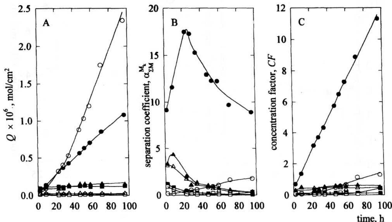
Fig. 4. Transport properties of the CME system with Acorga P-50: (A) cumulative stripping curves, (B) overall separation coefficients, (C) concentration factors; (●) Zn, (○) Cu, (■) Ca, (□) Mg, (▲) Na, (△) K.
