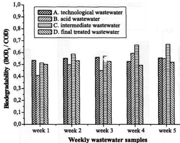
Fig. 4. Relative biodegradability of wastewater. Each of the results shown is represented by a mean value of 3 samples taken each week for 5 weeks.
