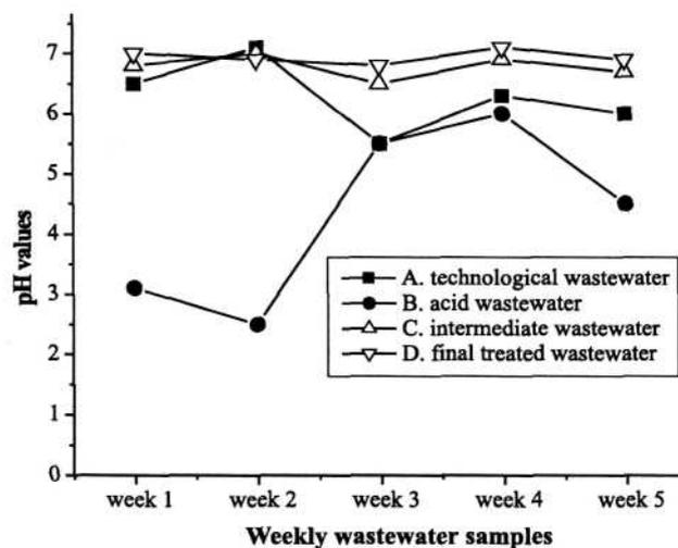
Fig. 3. Variations of wastewater pH values. Each of the results shown is represented by a mean value of 3 samples taken each week for 5 weeks.
