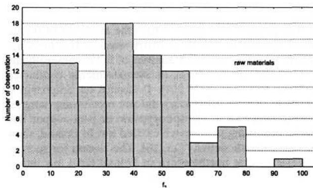
Fig. 2b. Variety of qualifying coefficients  $f_2$  for raw materials.
