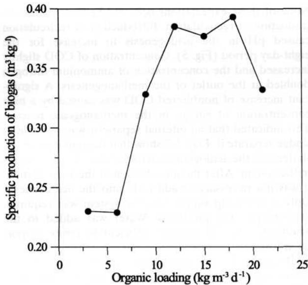
Fig. 8. Specific production of biogas at individual OLR of the methanogenic reactor.
