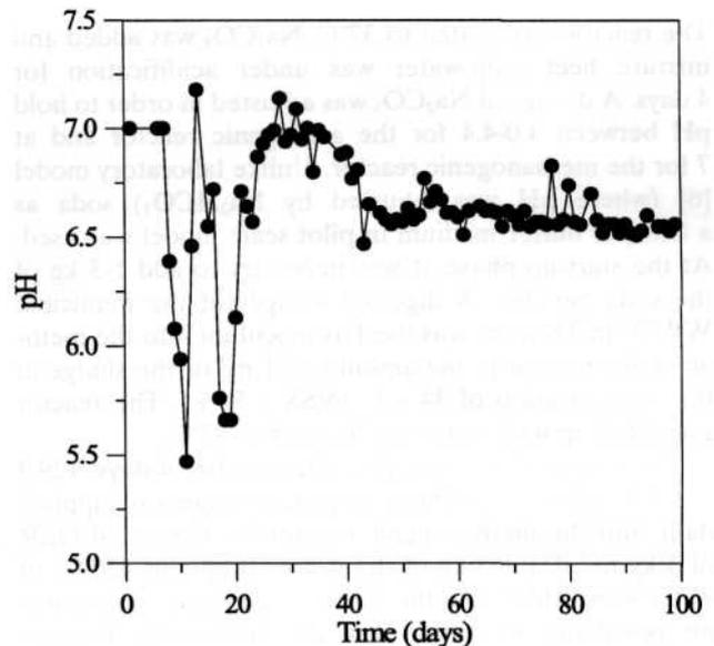
Fig. 6. pH in methanogenic reactor.
