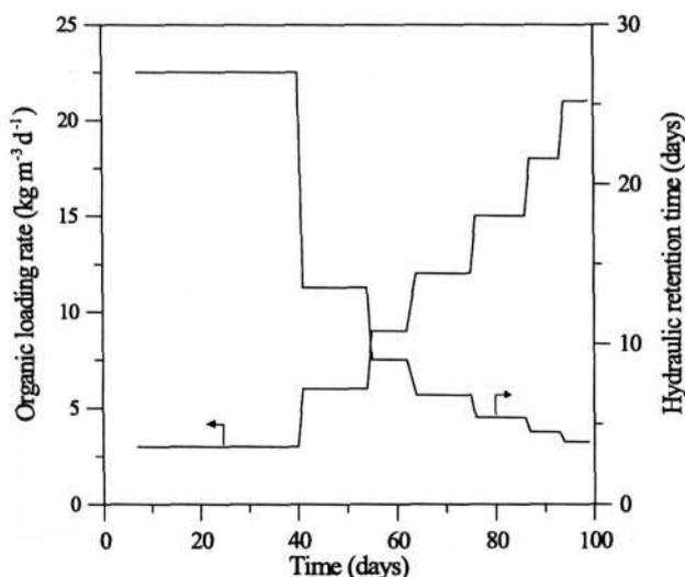
Fig. 2. Course of organic loading rate and hydraulic retention time in methanogenic reactor.
