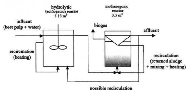
Fig. 1. Pilot-scale model of anaerobic treatment of sugar beet pulp.
