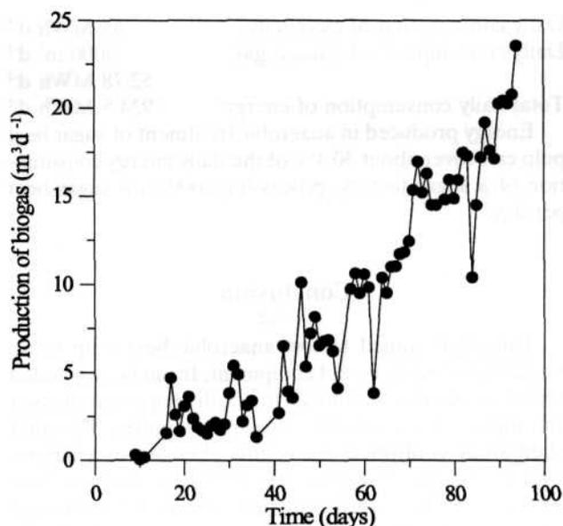
Fig. 7. Biogas production in methanogenic reactor.
