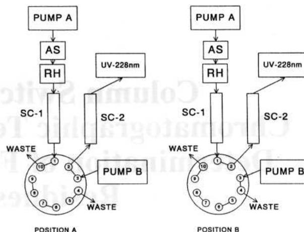
Fig. 1. Diagram of column switching liquid chromatographic system.
