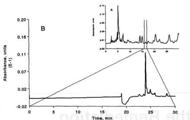
Fig. 4. The chromatogram of the sample extract on SC-1 clean-up column 1 coupled directly to UV-PDA detector (A) and the chromatogram of SC-1 effluent portion on SC-2 analytical column 2 (B). The fenoxycarb peak is identified by its retention time (24.1 min).
