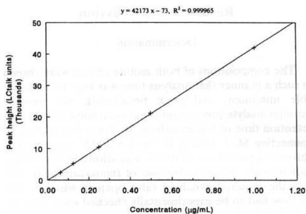
Fig. 2. Peak height calibration over concentration range 0.06 - 1.00  $\mu\text{g/mL}$  for fenoxycarb.
