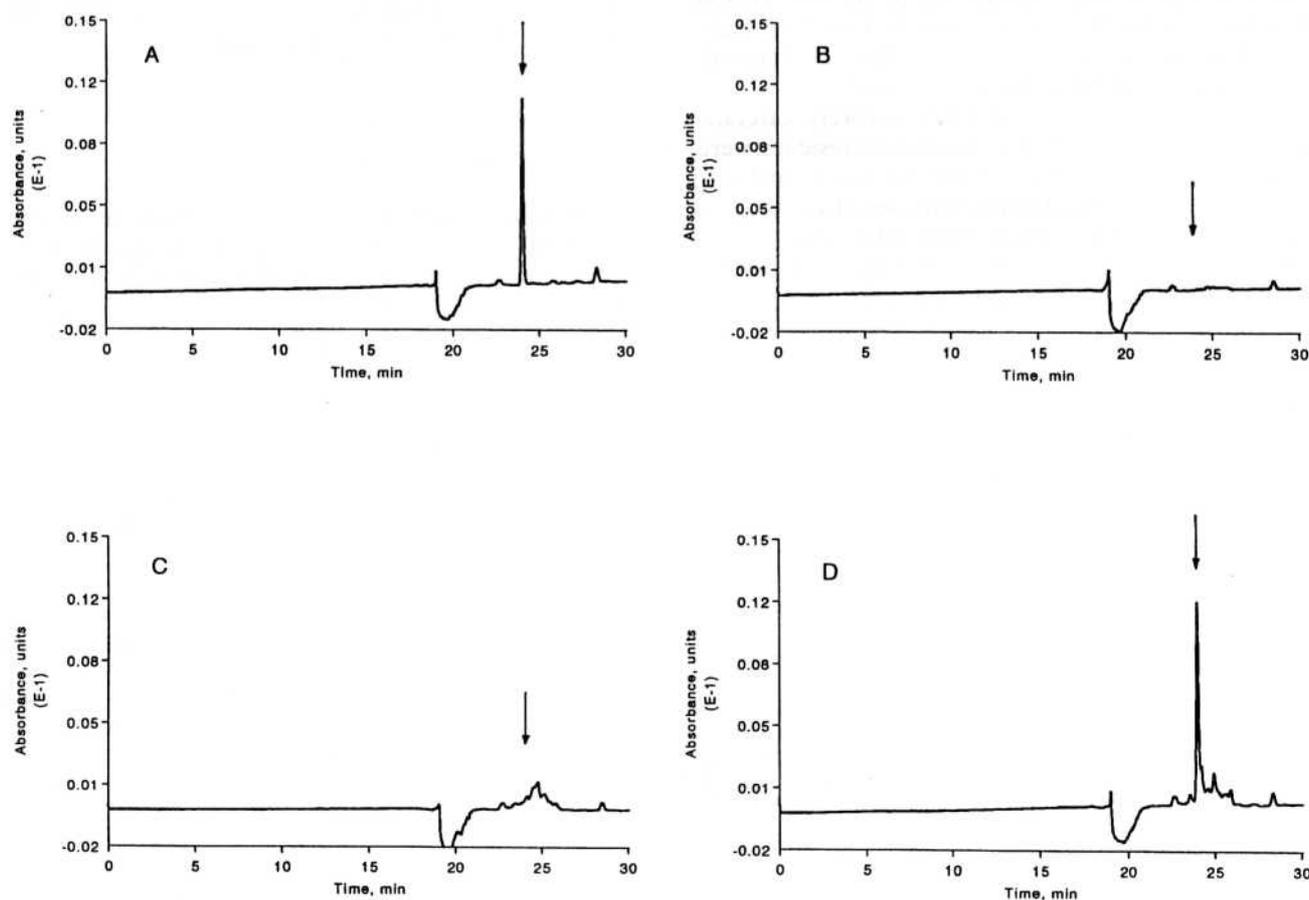
Fig. 3. Typical chromatograms (arrow indicates fenoxycarb): (A) - fenoxycarb standard 0.2  $\mu\text{g/mL}$ ; (B) - reagent blank; (C) - 5 g untreated control apples; (D) - 5 g control apples fortified at 0.1 mg/kg (80.9% recovery).
