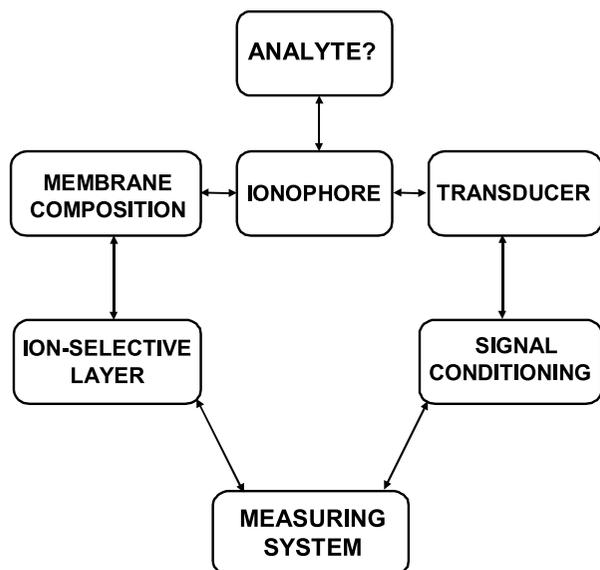
Fig. 4. Steps in the design of a potentiometric chemical sensor.
