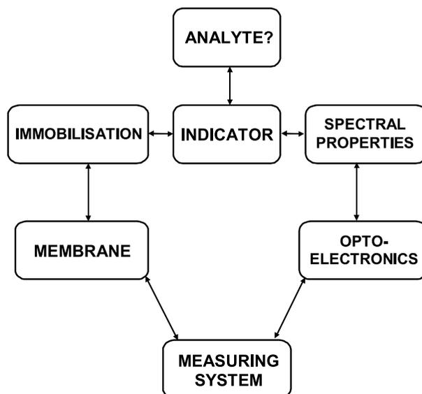
Fig. 5. Steps in design of a fibre optic chemical sensor.
