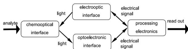
Fig. 2. Signal conversion in a fibre optic chemical sensor.
