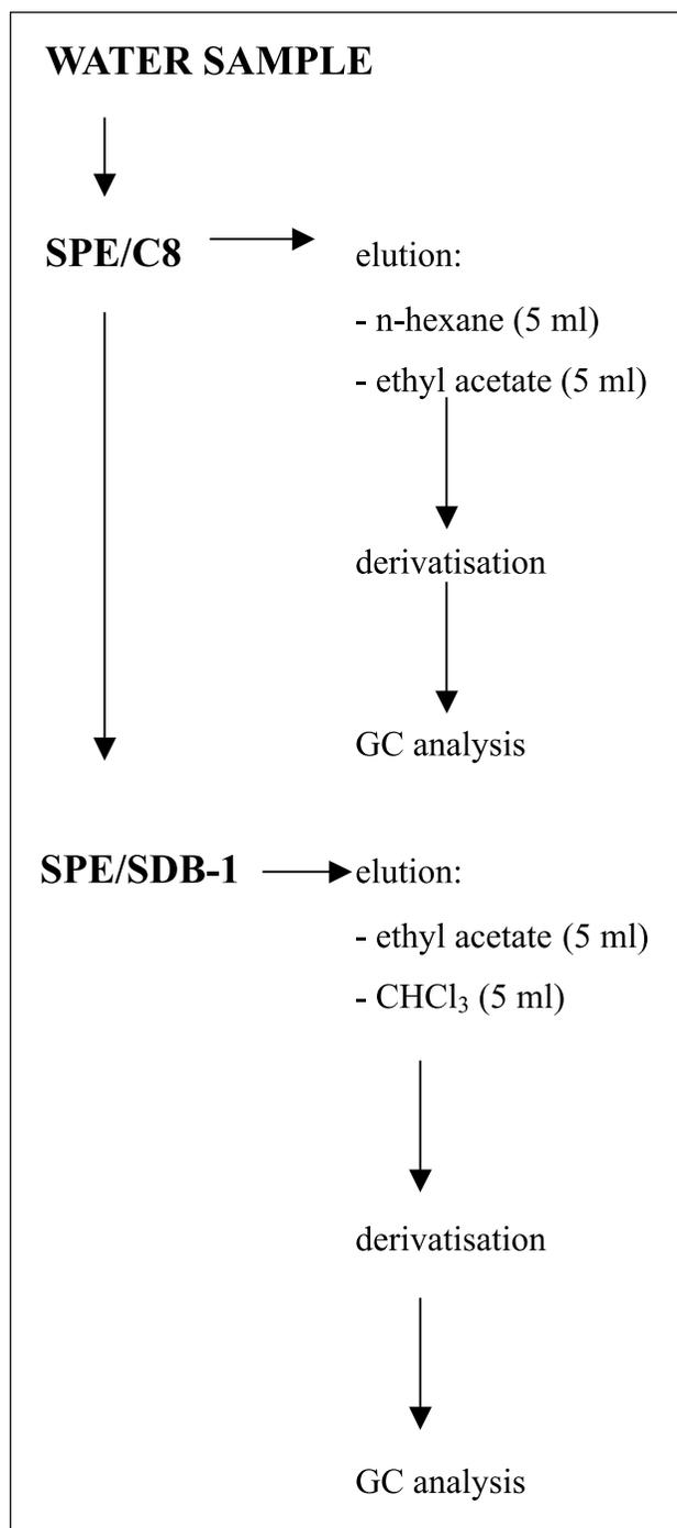
Fig. 1. The SPE procedure [15].
