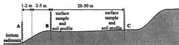
Fig. 2. Scheme of sediment and soil collection sites.
