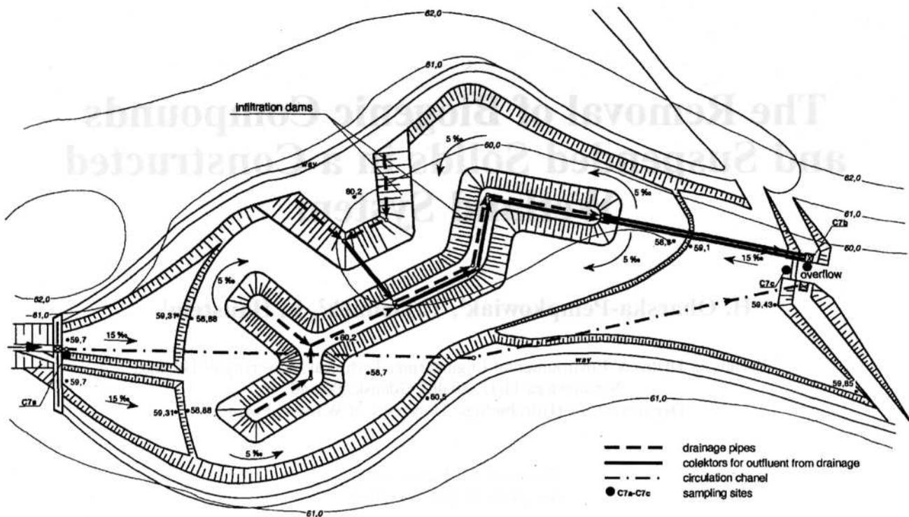
Fig. 1. The schematic of constructed wetland system in Bielkowo.
