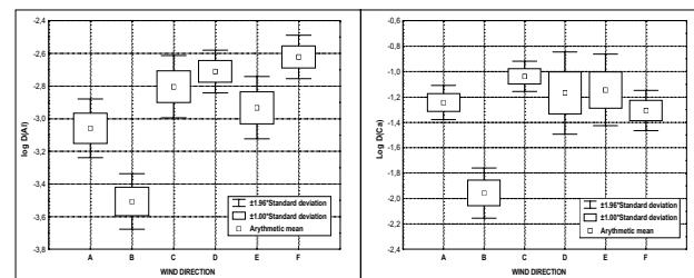
Fig. 9. Dependence of parameters  $\log D(\text{Al}^{3+})$  and  $\log D(\text{Ca}^{2+})$  on the direction of air advection (precipitation related to all six types of wind direction).
