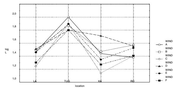
Fig. 6. Electrolytic conductivity parameters  $\log L$  [ $\mu\text{S}$ ] for different sampling site categories and wind direction types.
