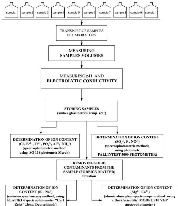
Fig. 2. Schematic presentation of analytical procedure for precipitation water samples.
