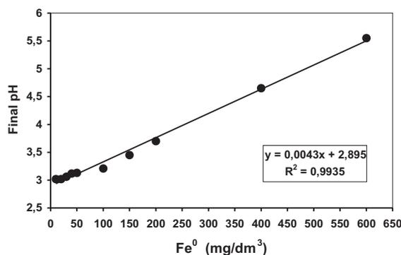
Fig. 6. Effect of iron powder dosage on final pH (60 mg H<sub>2</sub>O<sub>2</sub>/dm<sup>3</sup>; pH = 3,0).
