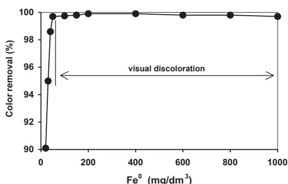
Fig. 4. Effect of  $\text{Fe}^0$  amount on color removal by  $\text{H}_2\text{O}_2/\text{Fe}^0$  process ( $\text{H}_2\text{O}_2 = 60 \text{ mg/dm}^3$ ; 3.0 pH).
