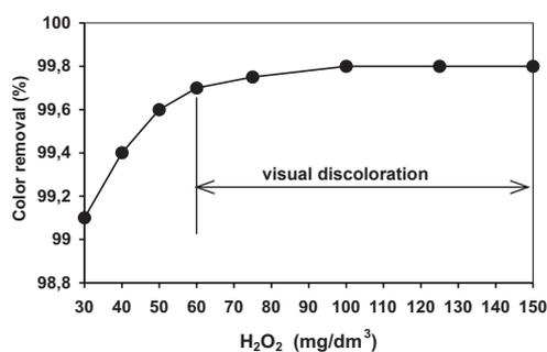
Fig. 2. Effect of  $\text{H}_2\text{O}_2$  dosage on color removal by  $\text{H}_2\text{O}_2/\text{Fe}^0$  process ( $\text{Fe}^0 = 1 \text{ g/dm}^3$ ; 3.5 pH).
