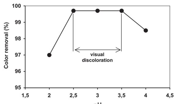
Fig. 3. Effect of pH on color removal by  $\text{H}_2\text{O}_2/\text{Fe}^0$  process ( $\text{Fe}^0 = 1 \text{ g/dm}^3$ ;  $\text{H}_2\text{O}_2 = 60 \text{ mg/dm}^3$ ).
