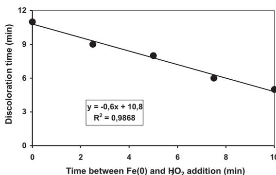
Fig. 7. Effect of time between Fe<sup>0</sup> and H<sub>2</sub>O<sub>2</sub> addition on discoloration time (pH = 3,0; 60 mg H<sub>2</sub>O<sub>2</sub>/dm<sup>3</sup>; Fe<sup>0</sup> = 200 mg/dm<sup>3</sup>).
