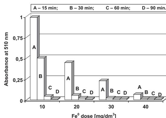
Fig. 5. Effect of reaction time on color removal by H<sub>2</sub>O<sub>2</sub>/Fe<sup>0</sup> process (H<sub>2</sub>O<sub>2</sub> = 60 mg/dm<sup>3</sup>; 3.0 pH).
