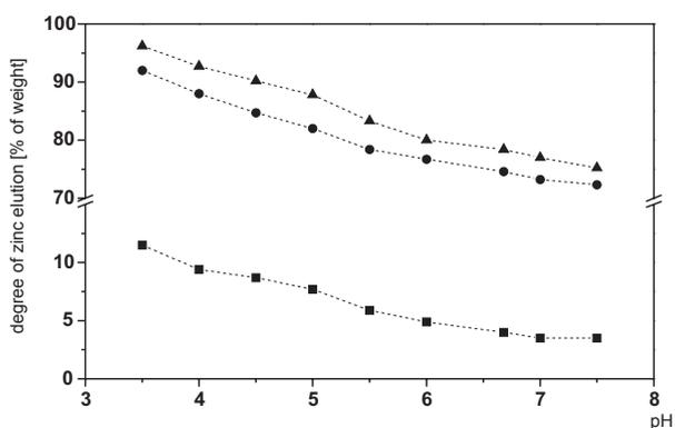
Fig. 5. Comparison of the degree of zinc elution from a sample of sludge stabilized by quicklime, cement kiln dust and detrital basalt OW13 B20 with a sample of post-digestion sludge, and from a sample of OW13 (post-digestion sludge after mixing with minced willow twigs at weight ratio d.m. 1:3).
