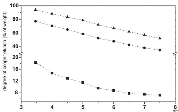
Fig. 4. Comparison of the degree of copper elution from a sample of sludge stabilized by quicklime, cement kiln dust and detrital basalt OW13 B20 with a sample of post-digestion sludge, and from a sample of OW13 (post-digestion sludge after mixing with minced willow twigs at weight ratio d.m. 1:3).
