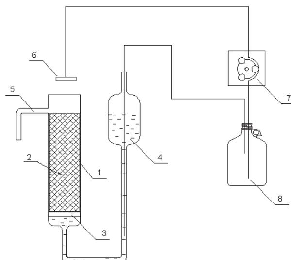
Fig. 2. Scheme of the system used to determine the degree of heavy metals elution from samples using the continuous method. 1 - glass container for eluting, 2 - sludge sample, 3 - glass sinter, 4 - overflow tank, 5 - nozzle, 6 - sprinkler, 7 - peristaltic pump, 8 - solution tank.
