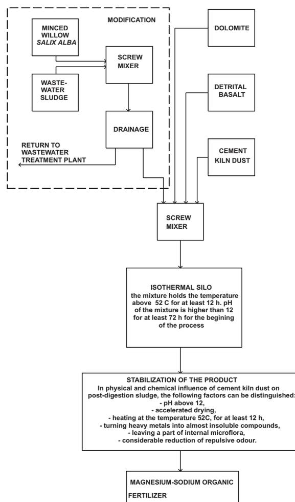
Fig. 1. Scheme of modification of wastewater sludge hygienization.
