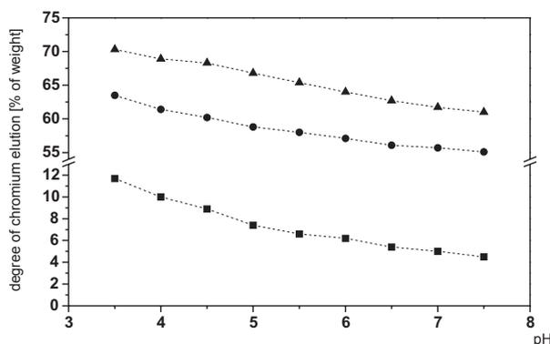
Fig. 6. Comparison of the degree of chromium elution from a sample of sludge stabilized by quicklime, cement kiln dust and detrital basalt OW13 B20 with a sample of post-digestion sludge, and from a sample of OW13 (post-digestion sludge after mixing with minced willow twigs at weight ratio d.m. 1:3).
