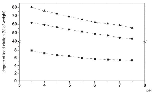
Fig. 3. Comparison of the degree of lead elution from a sample of sludge stabilized by quicklime, cement kiln dust and detrital basalt OW13 B20 with a sample of post-digestion sludge, and from a sample of OW13 (post-digestion sludge after mixing with minced willow twigs at weight ratio d.m. 1:3).
