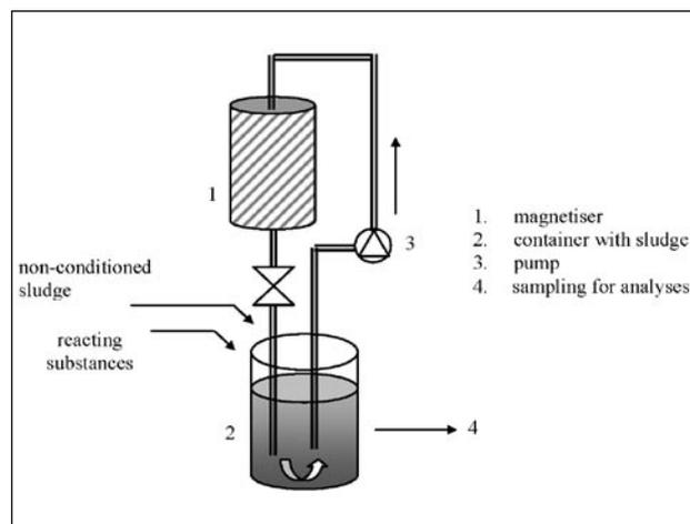
Fig. 2. Experimental stand in phase II (dynamic method).
