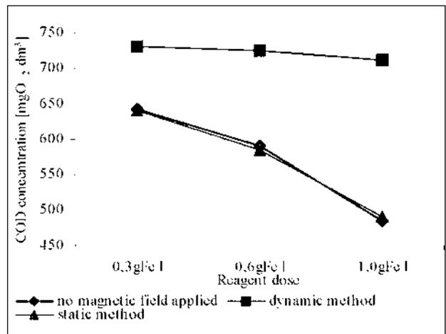
Fig. 9. Iron chloride impact on COD.
