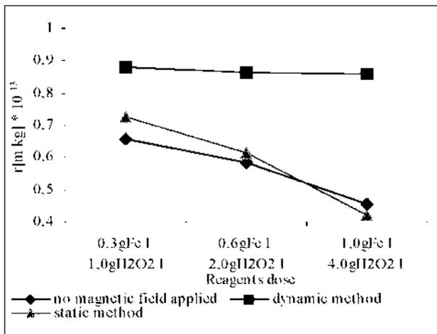
Fig. 6. Fenton's reagent impact on specific filtration resistance.
