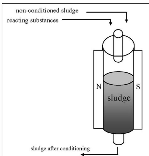
Fig. 3. Experimental stand in phase III (static method).
