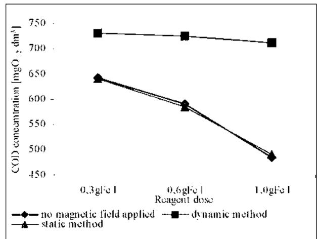
Fig. 9. Iron chloride impact on COD.
