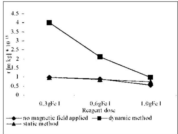
Fig. 8. Iron chloride impact on specific filtration resistance.
