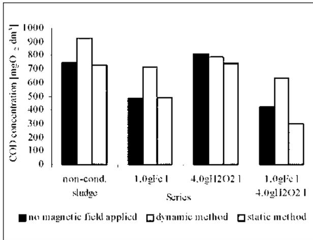
Fig. 5. Magnetic field impact on COD, at the highest doses of reacting substances.
