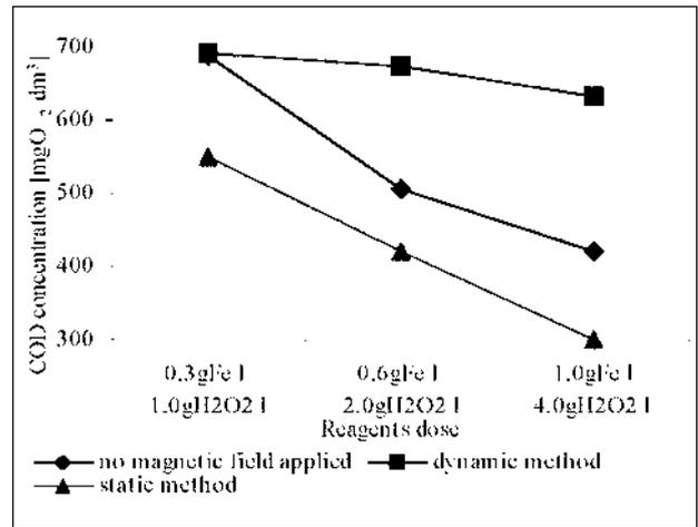
Fig. 7. Fenton's reagent impact on COD.
