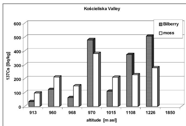
Fig.1a. The dependence of  $^{137}\text{Cs}$  activity ( Bq/kg) on altitude formoss and bilberry samples taken from Kościeliska Valley region .
