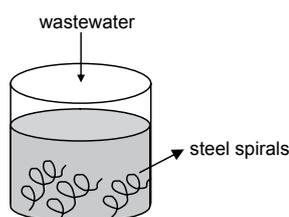
Fig. 1. Scheme of the experimental post in the first stage of the experiment with steel packing using.
