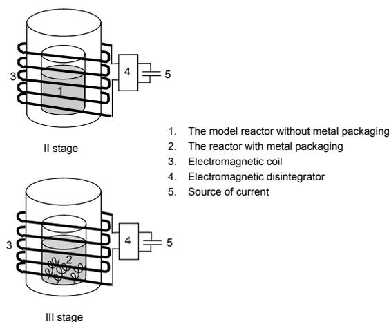
Fig. 2. Scheme of the experimental post in the second and third stage of the experiment.
