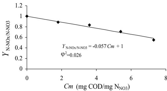
Fig. 6. The ratio between denitrification rate and nitrate reduction rate ( $Y_{N-NO_x/N-NO_3}$ ) versus methanol dosage ( $C_m$ ).
