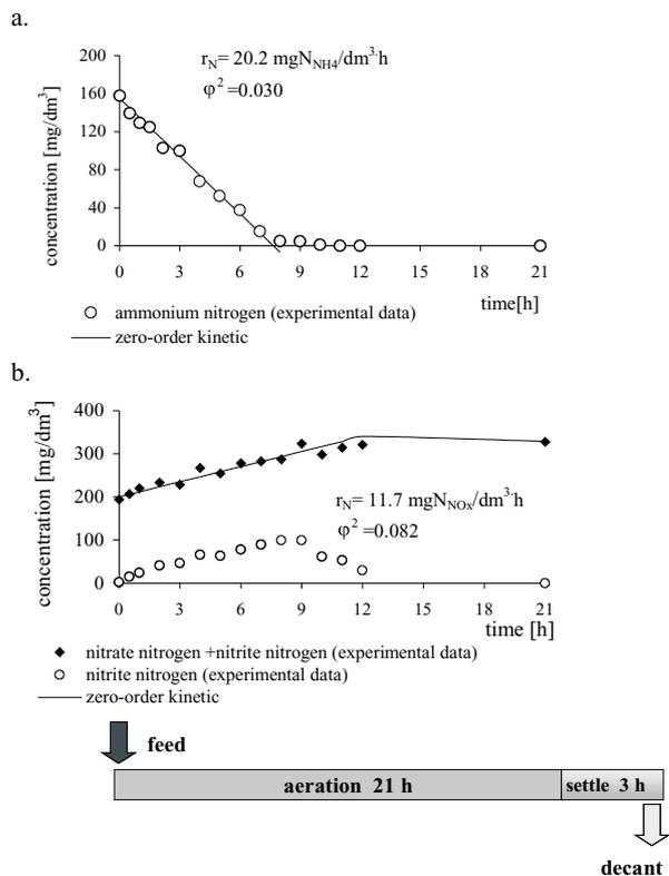
Fig. 2. Concentrations profiles in leachate of ammonium nitrogen (a), nitrate nitrogen and nitrite nitrogen (b) during aerobic conditions and reaction rates described by zero-order kinetics at HRT 2d (SBR 2-N).
