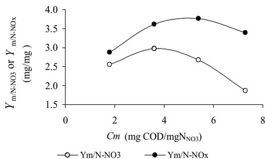
Fig. 7. Yield methanol coefficients ( $Y_{m/N-NO_3}$  and  $Y_{m/N-NO_x}$ ) versus methanol dosage ( $C_m$ ).
