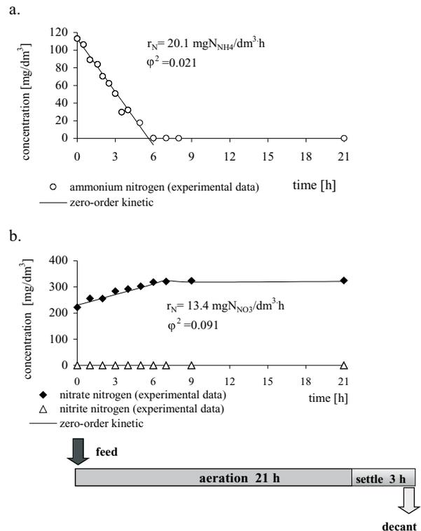
Fig. 1. Concentrations profiles in leachate of ammonium nitrogen (a), nitrate nitrogen and nitrite nitrogen (b) during aerobic conditions and reaction rates described by zero-order kinetics at HRT 3d (SBR 1-N).
