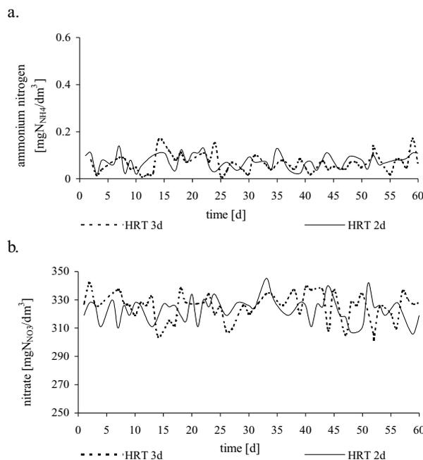
Fig. 4. Concentration of ammonium nitrogen (a) and nitrate nitrogen (b) in the effluent from SBR reactors (steady conditions).
