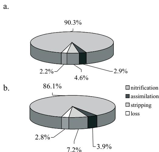
Fig. 3. Ammonium nitrogen balance during SBR reactor operating cycle; a. SBR 1-N (HRT 3d) b. SBR 2-N (HRT 2d).
