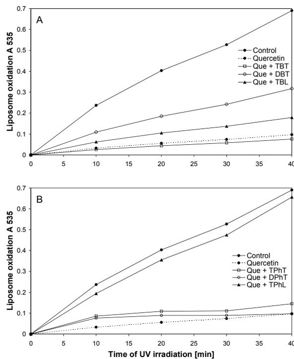
Fig. 2. Liposome oxidation levels of PC membranes induced by quercetin and its equimolar mixtures with butyl tin and lead compounds (A) and phenyl tin and lead compounds (B) as a function of UV irradiation time. Standard deviation was studied  $\leq 0.04$ .
