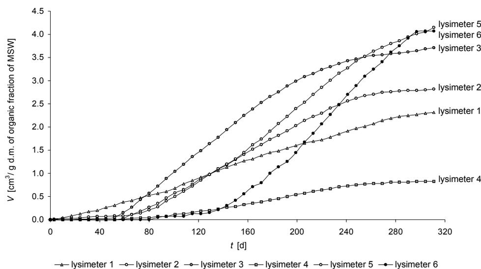
Fig. 2. Cumulative landfill gas production in lysimeters during the 311 days of the experiment.
