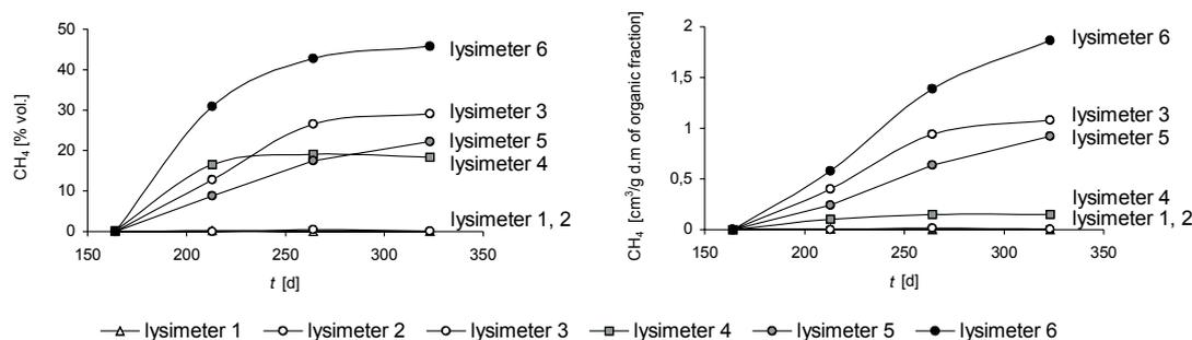
Fig. 4. Methane production in lysimeters during 311 days of the experiment.
