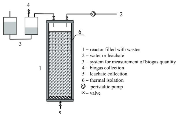
Fig. 1. The scheme of the research station.
