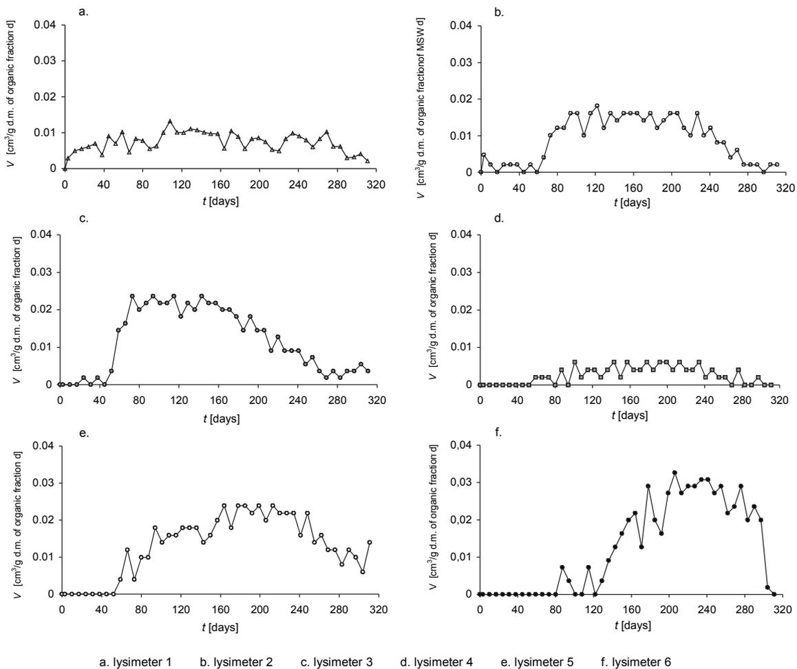
Fig. 3. Daily amount of produced biogas during 311 days of the experiment.
