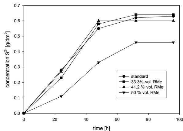
Fig. 4. The effect of RMe concentration on the kinetics of desulfurication taking place with the use of the *Desulfotomaculum ruminis* bacteria (C/S = 1.8, 37°C).
