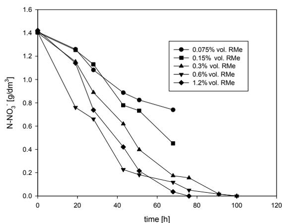
Fig. 1. The effect of the content of RMe on the process of denitrification carried out with the use of the *Bacillus licheniformis* bacteria (pH = 8, 22°C).
