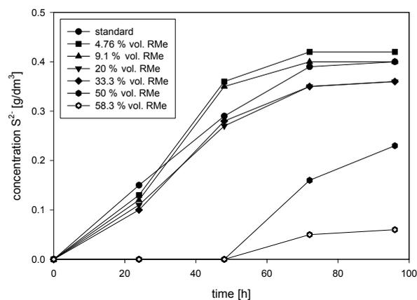
Fig. 3. The effect of RMe concentration on the kinetics of desulfurication taking place with the use of the *Desulfotomaculum ruminis* bacteria, (C/S = 0.9, 37°C).
