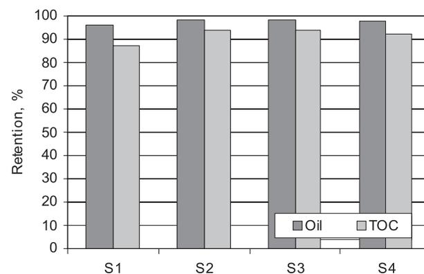
Fig. 4. Retention of oil and TOC in UF process for various feeds (at constant 0.2MPa transmembrane pressure). Feed: the content of oil in the feed: S1 – 100 ppm of oil, S2 – 200 ppm of oil, S3 – 300 ppm of oil, S4 – 400 ppm of oil.
