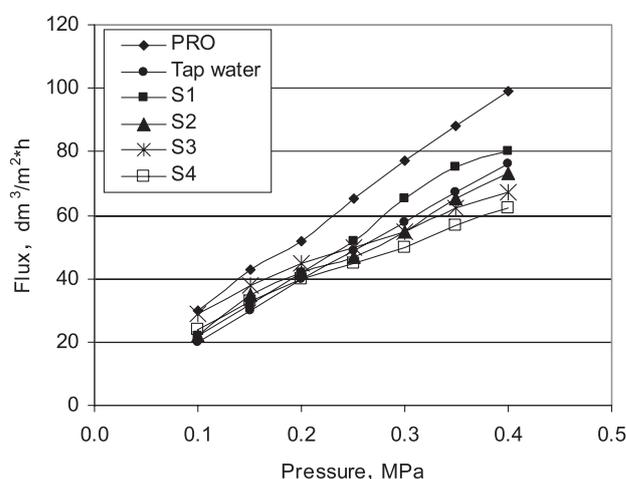
Fig. 3. Determination of the transport properties of UF membranes. The influence of the transmembrane pressure on the permeate flux. Feed: PRO – permeate RO, Tap water, S1 – 100 ppm of oil, S2 – 200 ppm of oil, S3 – 300 ppm of oil, S4 – 400 ppm of oil.
