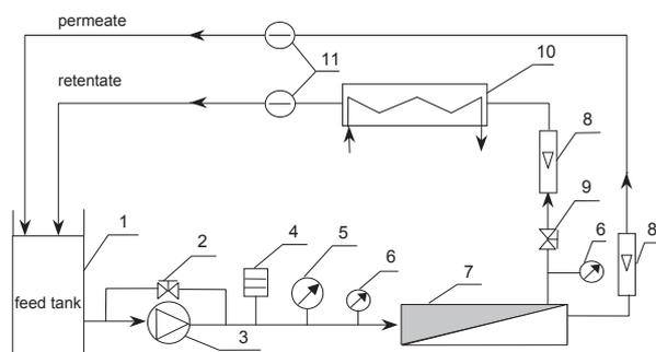
Fig. 1. Scheme of NF/UF pilot plant; 1 – feed tank, 2 – by-pass valve, 3 – pump, 4 - dampener, 5 – pressure gauge, 6 – manometer, 7 – module, 8 – rotameter, 9 – throttling valve, 10 – heat exchanger, 11 – control of temperature, conductivity.
