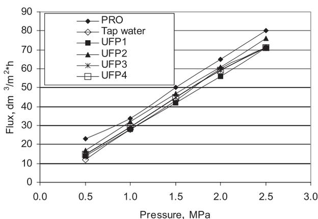
Fig. 5. The influence of transmembrane pressure on the permeate flux: Feed: UFP1 – UF permeate from series 100 ppm of oil, UFP2 – UF permeate from series 200 ppm of oil, UFP3 – UF permeate from series 300 ppm of oil, UFP4 – UF permeate from series 400 ppm of oil.
