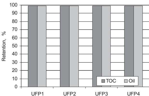
Fig. 6. Retention of oil and TOC in the NF process at constant pressure (1.0 MPa). Feed: UFP1 – UF permeate from series 100 ppm of oil, UFP2 – UF permeate from series 200 ppm of oil, UFP3 – UF permeate from series 300 ppm of oil, UFP4 – UF permeate from series 400 ppm of oil.
