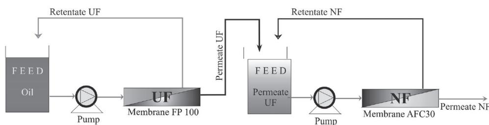
Fig. 2. Flow sheet of the UF/NF system for the removal of oil from wastewater.
