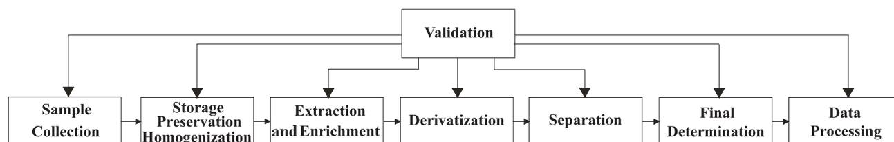
Fig. 1. Operations and processes used during preparation of samples of sediments and soils for the determination of organometallic compounds.
