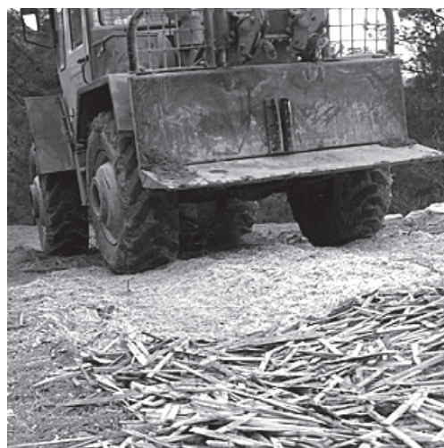
Fig. 1. A rubber-tired skidder (MB Trac 900) traveling on slash treatments.
