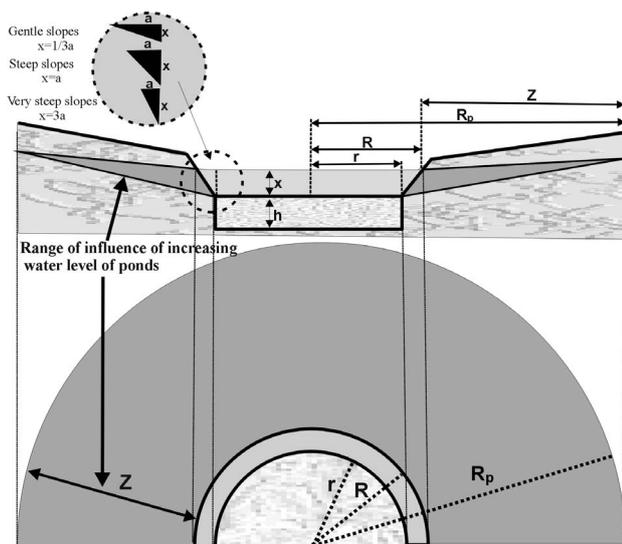
Fig. 2. Scheme used for the calculation of changes of pond and groundwater retention as a result of water level increase in a pond ( $r$  – a pond radius before water damming;  $R$  – a pond radius after water damming;  $R_p$  – a radius of an area where the increase of groundwater retention is observed;  $x$  – the height of water damming in a pond;  $Z$  – the range of impact of water damming;  $h$  – average depth of water in a pond
