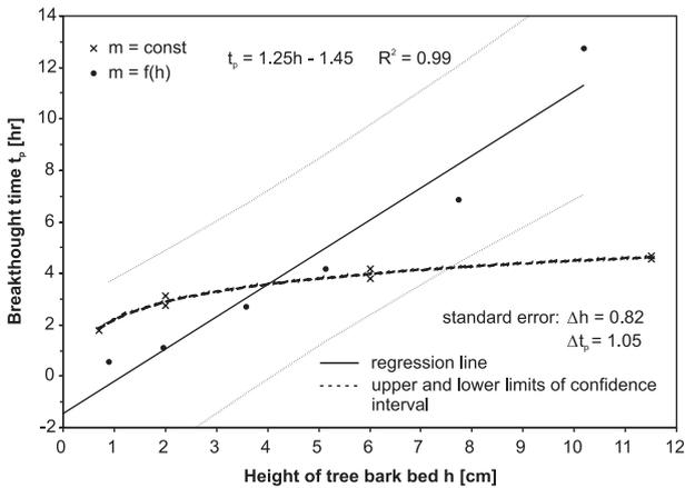
Fig. 6. A relationship between breakthrough time ( $t_p$ ) and bark bed height ( $h$ ) for ammonia concentration  $1.40\text{mg}/\text{dm}^3$  in the  $\text{NH}_3/\text{air}$  mix and flow intensity  $Q=1\text{dm}^3/600\text{s}$
