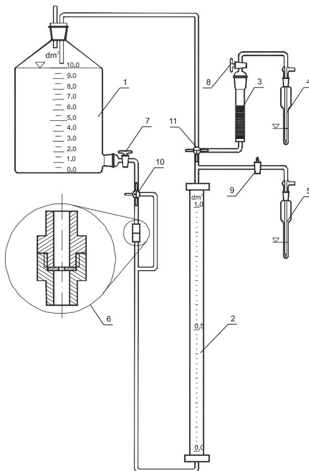
Fig. 2. A schematic of the measuring set-up: 1- holding vessel for aqueous ammonia solution; 2- dispenser of  $1\text{dm}^3$  portions of gaseous ammonia; 3- adsorption column filled with tree bark; 4 and 5- sulfuric acid scrubbers (Polezajew type gas-washing bottles); 6- controllable flow nozzle; 7-9- cut-off valves; 10 and 11 – two 2/3-way valves
