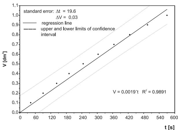
Fig. 4. Flow dynamics of the ammonia/air mix passing through the studied adsorbant bed at  $\mathcal{Q}=1\text{dm}^3/600\text{s}$ .
