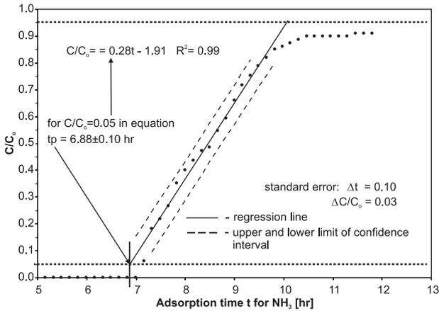
Fig. 5. Estimation of breakthrough time  $t_p$  for the “ammonia/tree bark” adsorption system (bark bed height  $h=80\text{mm}$ )
