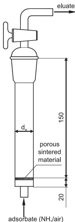
Fig. 3. Adsorption column ( $d_w = 16; 22; 35$  and  $60$ mm).
