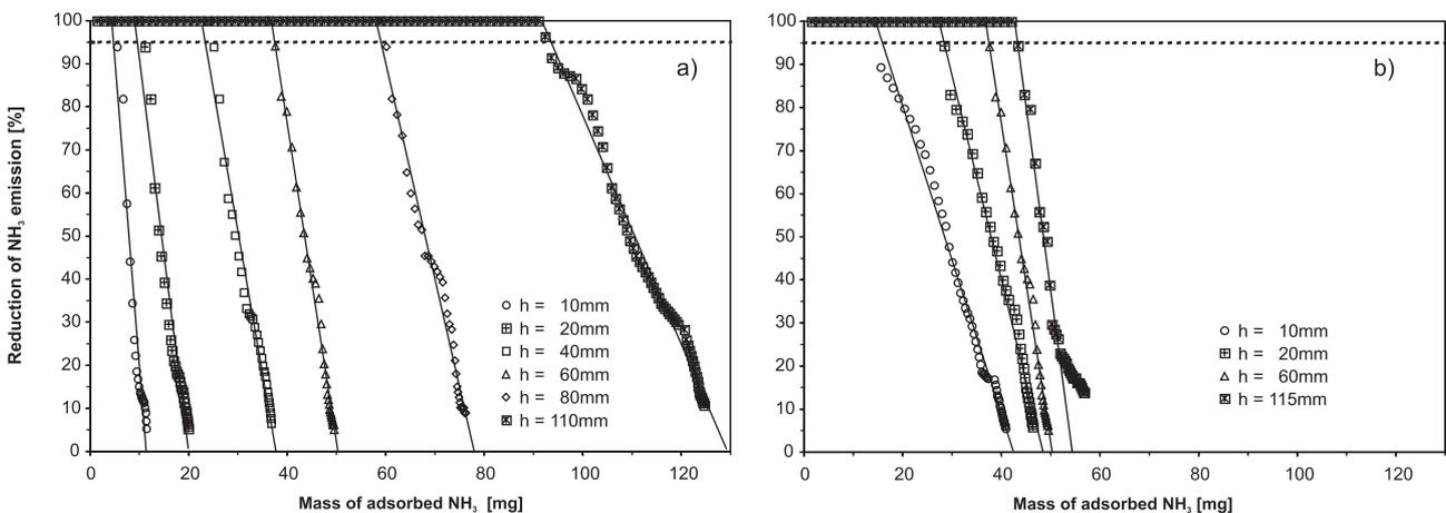
Fig. 7. Reduction of ammonia emission as a function of the mass of gas adsorbed onto bark beds of different height  $h=10\div 115\text{mm}$ : a)  $m = f(h)$ , b)  $m = \text{const}$
