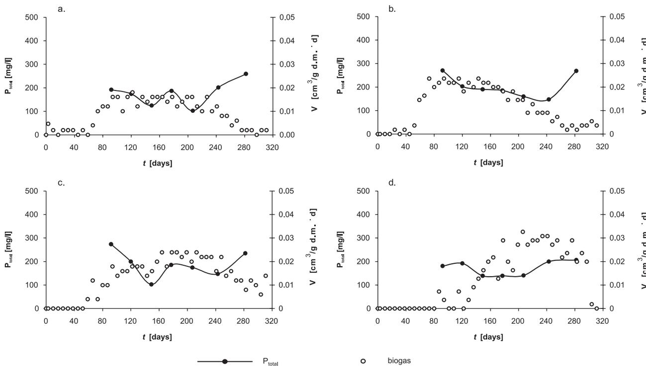
Fig. 6. Relationship between  $P_{\text{total}}$  concentration in leachate and biogas production. a – lysimeter 1, b – lysimeter 2, c – lysimeter 3, and d – lysimeter
