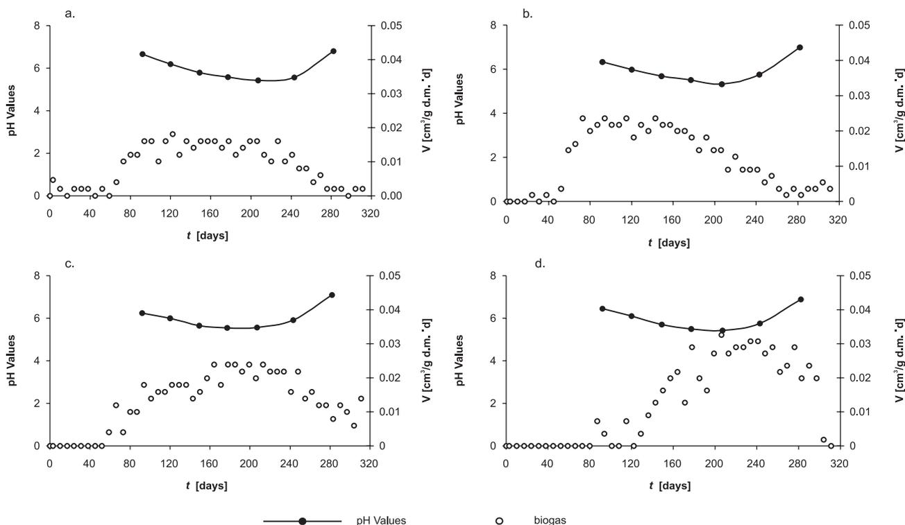
Fig. 8. Changes of leachate pH values over time. a – lysimeter 1, b – lysimeter 2, c – lysimeter 3, and d – lysimeter 4.
