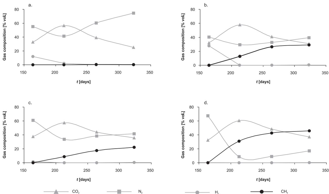
Fig. 7. Gas composition. a – lysimeter 1, b – lysimeter 2, c – lysimeter 3, and d – lysimeter 4.
