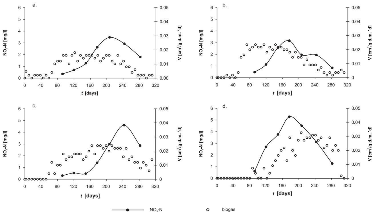
Fig. 5. Relationship between  $\text{NO}_3\text{-N}$  concentration in leachate and biogas production. a – lysimeter 1, b – lysimeter 2, c – lysimeter 3, and d – lysimeter.
