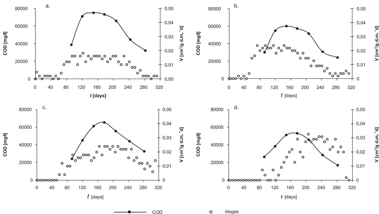
Fig. 2. Relationship between COD concentration in leachate and biogas production. a – lysimeter 1, b – lysimeter 2, c – lysimeter 3, and d – lysimeter 4.
