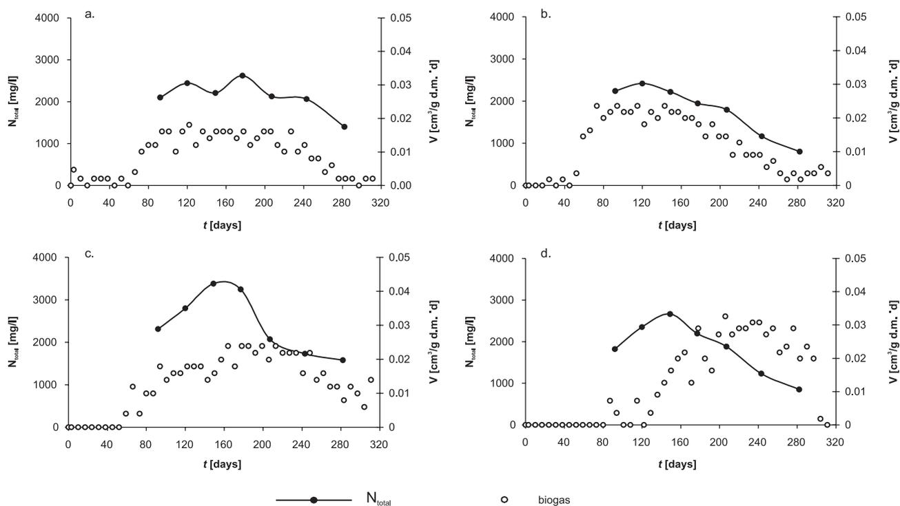
Fig. 3. Relationship between N-total concentration in leachate and biogas production. a – lysimeter 1, b – lysimeter 2, c – lysimeter 3, and d – lysimeter 4
